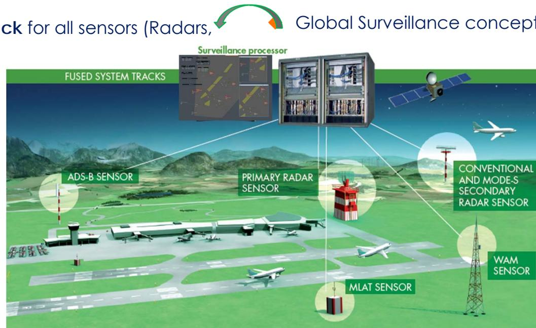
Radar, ADS-B, WAM Fused System Tracks
