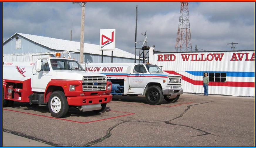
One of these fuel trucks is parked within 50 feet of a building that could provide an ignition source in the event of a fuel leak.
