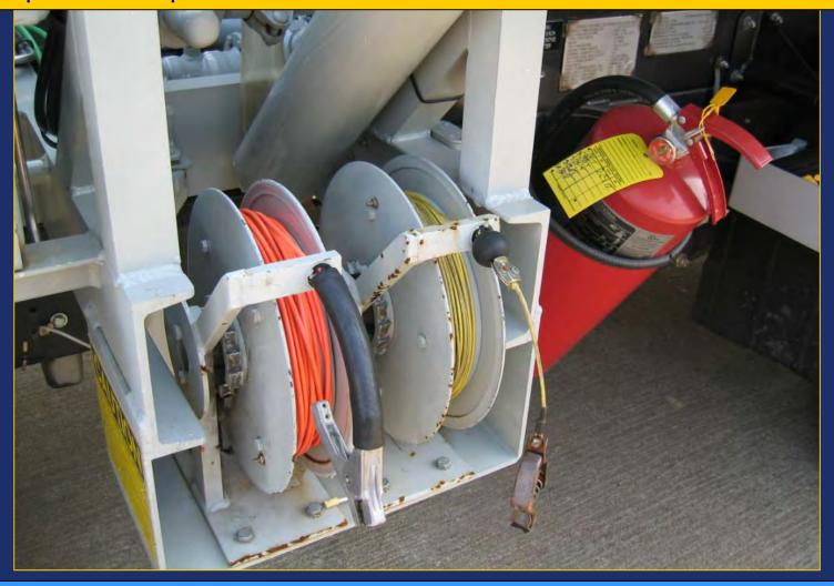
Bonding cables are required on fueling vehicles.
