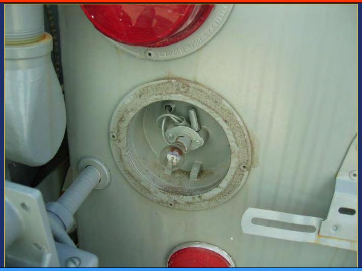
This missing tail light lens provides a potential ignition source.
