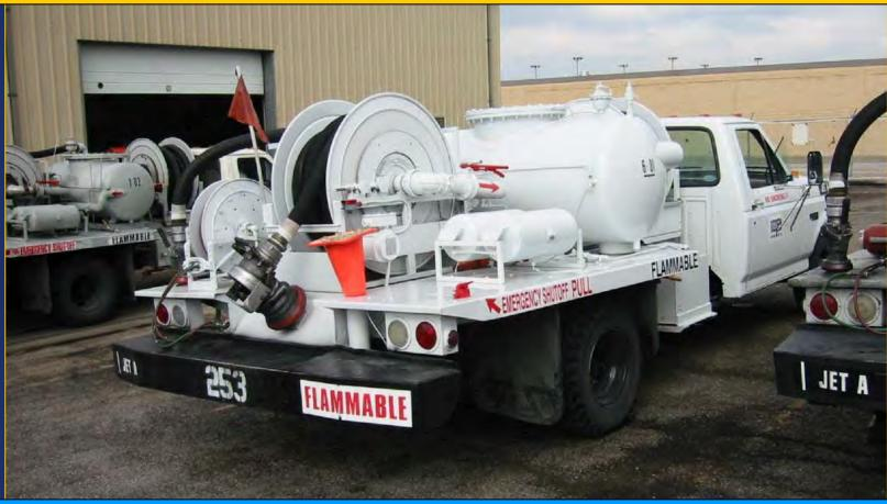
The fire code standard for parking 10 feet apart and at least 50 feet from buildings and aircraft does not apply for hydrant vehicles or carts because they do not carry much fuel.
