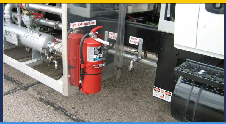
Two fire extinguisher are required on fuel servicing tank vehicles, with one mounted on each side.
