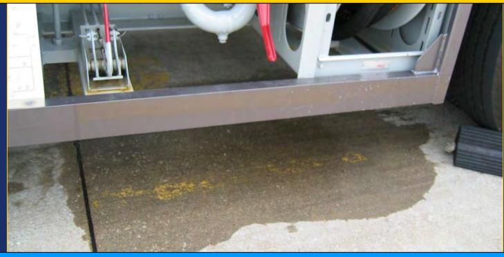
Most fuel leaks will have evidence of the leak on the pavement under the truck. Even when the truck is not present, fuel stains on the pavement will indicate leaking problems.
