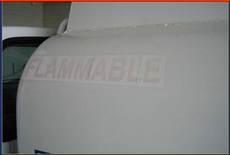
This FLAMMABLE sign is faded and not clearly visible.
