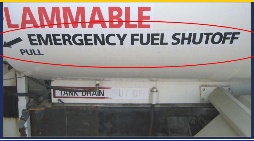
If both PUSH and PULL are on the placard, check the operation of the emergency shutoff to see if it is one way or the other. Some decal kits come with both PUSH and PULL labels to use, as appropriate, and the PUSH label needs to be removed on this truck. In addition, the placard is missing the "FUEL" portion of the EMERGENCY FUEL SHUTOFF placard.
