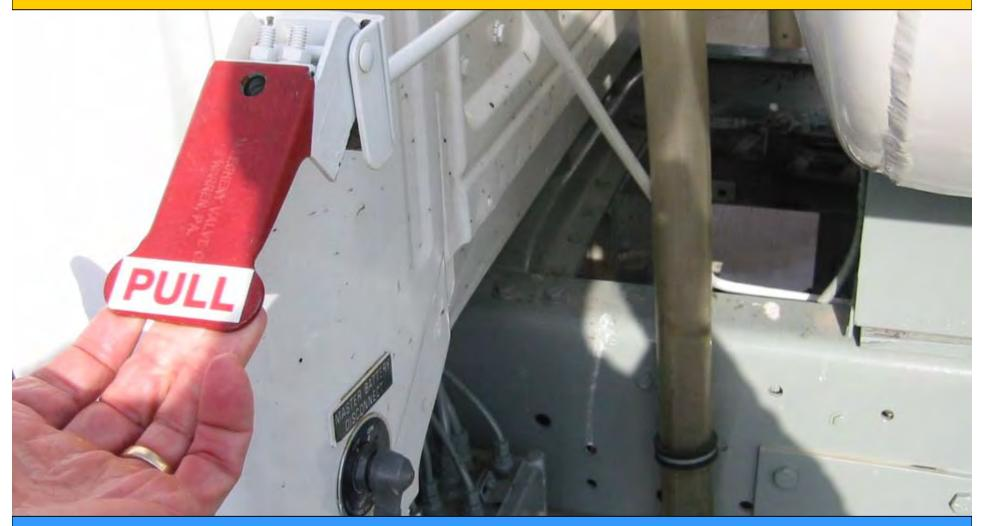
Ask fueling personnel what their procedure is for physically checking emergency fuel shutoff systems. Many fueling agents include a check of the emergency shutoff systems in their weekly or monthly checklists.
