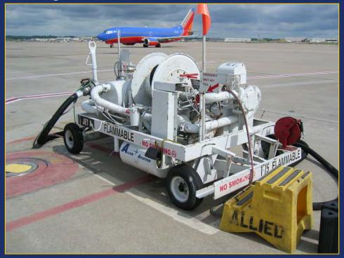
Aircraft fuel servicing carts are equipped with facilities to transfer fuel between a Airport Fueling System hydrant and an aircraft and are normally parked at a fixed location near a gate.
