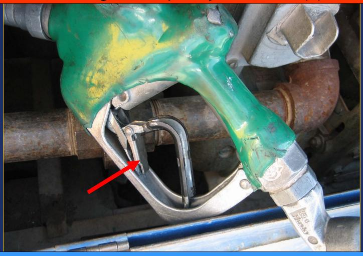
This nozzle has a latch system that allows bypassing the deadman control.
