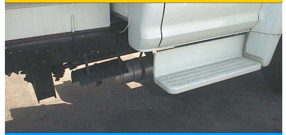
Any part of the engine exhaust system that extends out under the fuel tank or piping must be adequately shielded to prevent leaking fuel from dripping on the hot exhaust pipe.
