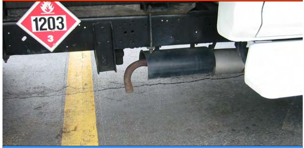
After the muffler was replaced with a longer muffler, the shielding is no longer adequate. Corrective action in this case was to shorten the exhaust pipe. The shield could also be extended in this situation.
