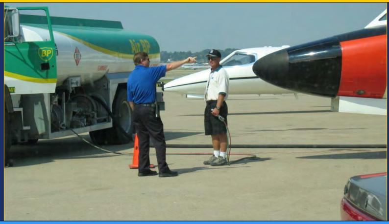
Observe fueling operations while inspecting aircraft fuel servicing vehicles to check for compliance with fire safety standards. In particular, check for proper bonding procedures and use of deadman controls.
