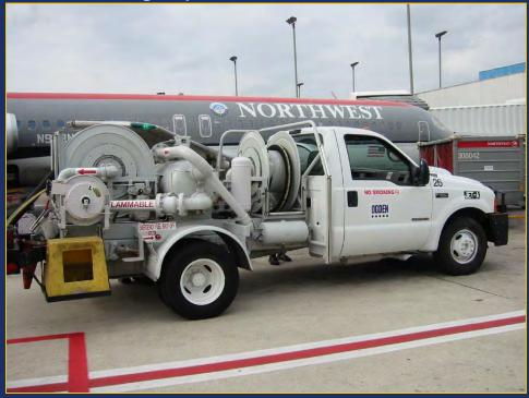
Aircraft fuel servicing hydrant vehicles are vehicles equipped with facilities to transfer fuel between an Airport Fueling System hydrant and an aircraft.
