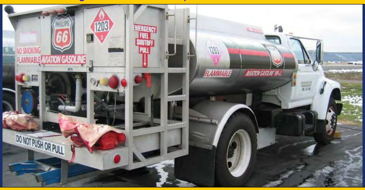
NFPA 407, Annex A Explanatory Material - A.5.13.5 Protection of Extinguishers Against Inclement Weather. During inclement weather, extinguishers not in enclosed compartments may be permitted to be protected by canvas or plastic covers. If icing occurs, the extinguisher should be sprayed with deicing fluid.
