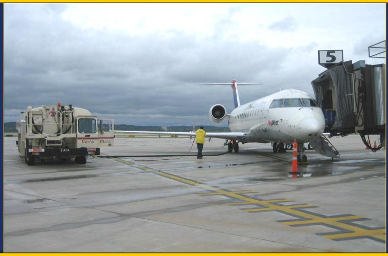
NFPA 407, 5.12.1 Aircraft fuel servicing vehicles and carts shall be positioned so that a clear path of egress from the aircraft for fuel servicing vehicles shall be maintained.
