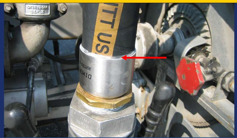
Check the coupling area of the hose for signs of hose slippage.
