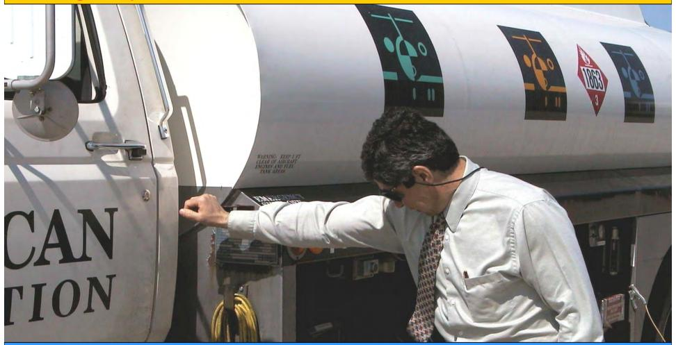
Physically activating the cable operated emergency shutoff systems when inspecting fuelers is highly recommended. Cable operated emergency shutoffs have problems with cables not being properly adjusted or being inoperable due to freezing or rust problems inside the cable sheaths.
