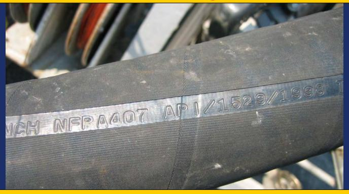
NFPA 407, 4.1.2.4 API BULL 1529, Aviation Fueling Hose, Type C hose (semiconductive) shall be used to prevent electrostatic discharges but shall not be used to accomplish required bonding. API BULL 1529, Type A hose that does not have a semiconductive cover shall not be used. Type F hose (hard wall) and Type CT hose (cold temperature) shall be permitted because they have semiconductive covers.
