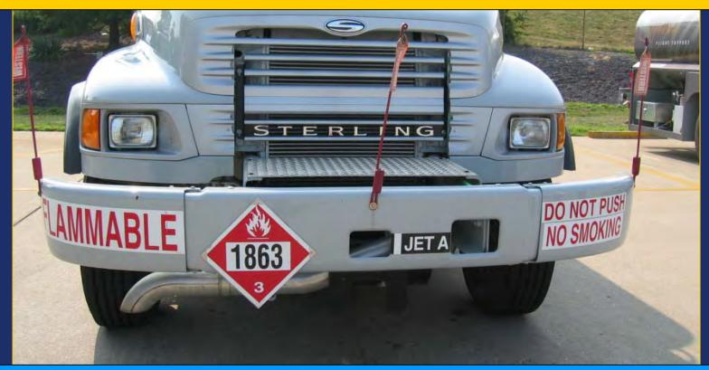
Most fuel trucks have the muffler and exhaust pipe at the front of the vehicle where it will be clear of fuel tanks and piping in the event of a leak.
