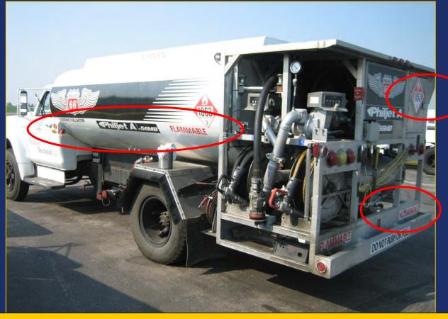
NFPA 407, 4.3.18 Each aircraft fuel servicing vehicle or cart shall have a sign on each side and the rear to identify the product. The sign shall have letters at least 3 inches (7.62 cm) high and shall be of a color contrasting sharply with the sign background for visibility. The word FLAMMABLE and the name of the product carried, such as JET A, JET B, GASOLINE, or AVGAS shall appear on the sign.
