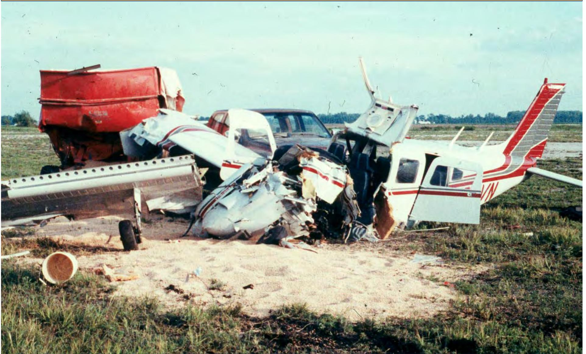
This incident occurred when a pilot lost control of the aircraft during takeoff and hit a grain trailer parked in the runway strip. 17
