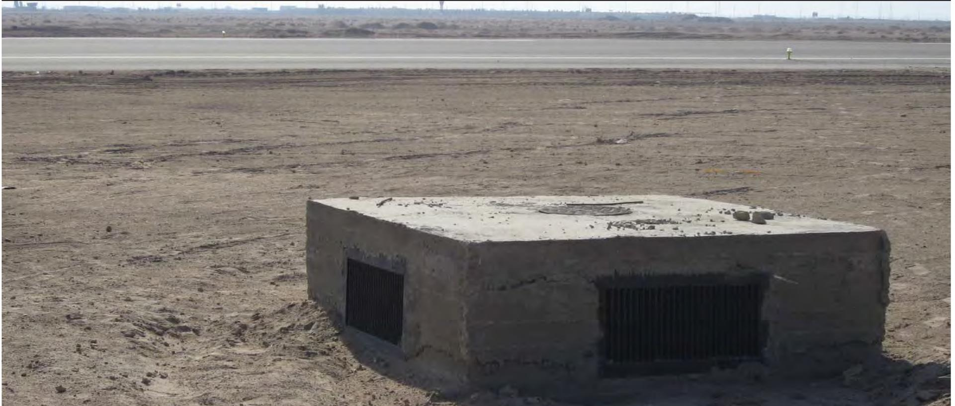
This large concrete structure provides a potentially hazardous situation in the event of an aircraft running off the runway.
