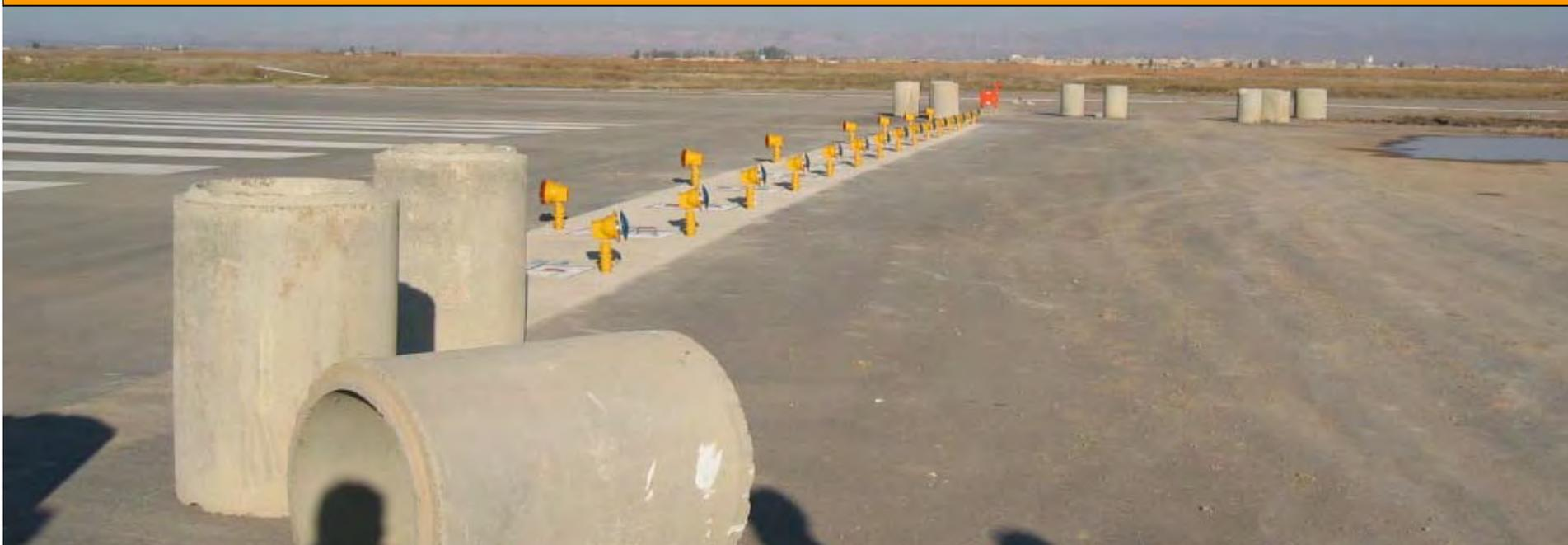
These concrete pipes are a significant hazard if hit by an aircraft and are located at the runway threshold where there is a higher risk of them being struck.
