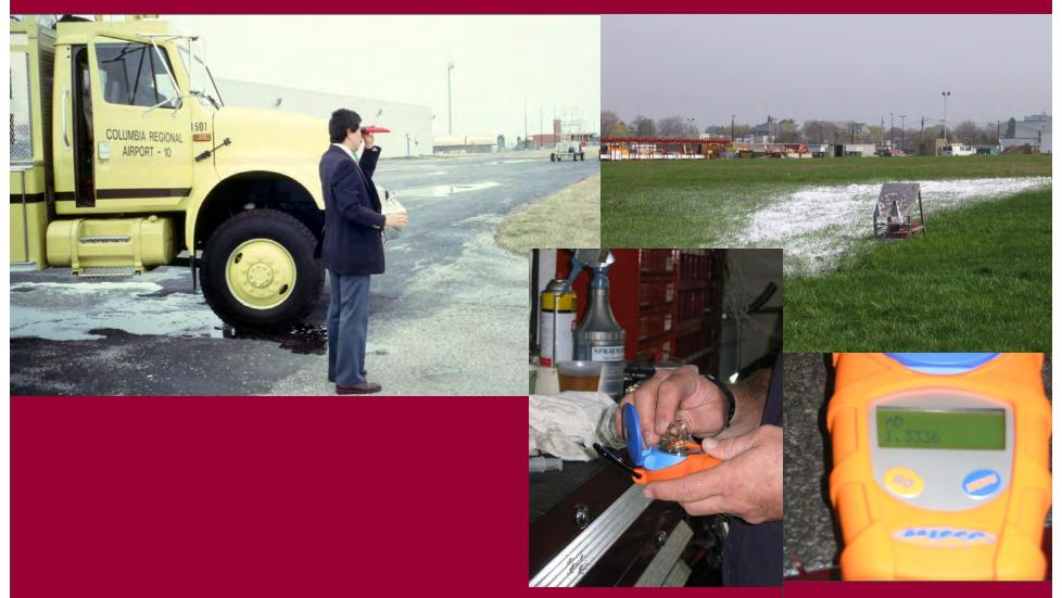
A test should be conducted by airport staff or ACSI if foam does not appear to be proportioned correctly
