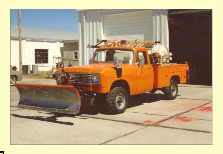
The ARFF vehicle has a plow mounted on the front
