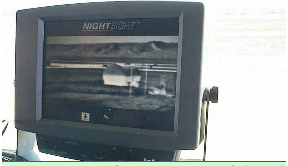
Flat screen type monitor mounted on dash in front of driver for better visibility while driving
