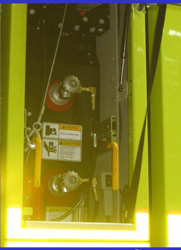
Check nitrogen tank gauges to ensure they are not discharged or below minimum pressure
