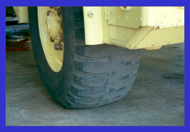
Check the condition of tires - worn tires provide poor traction in muddy off-pavement conditions
