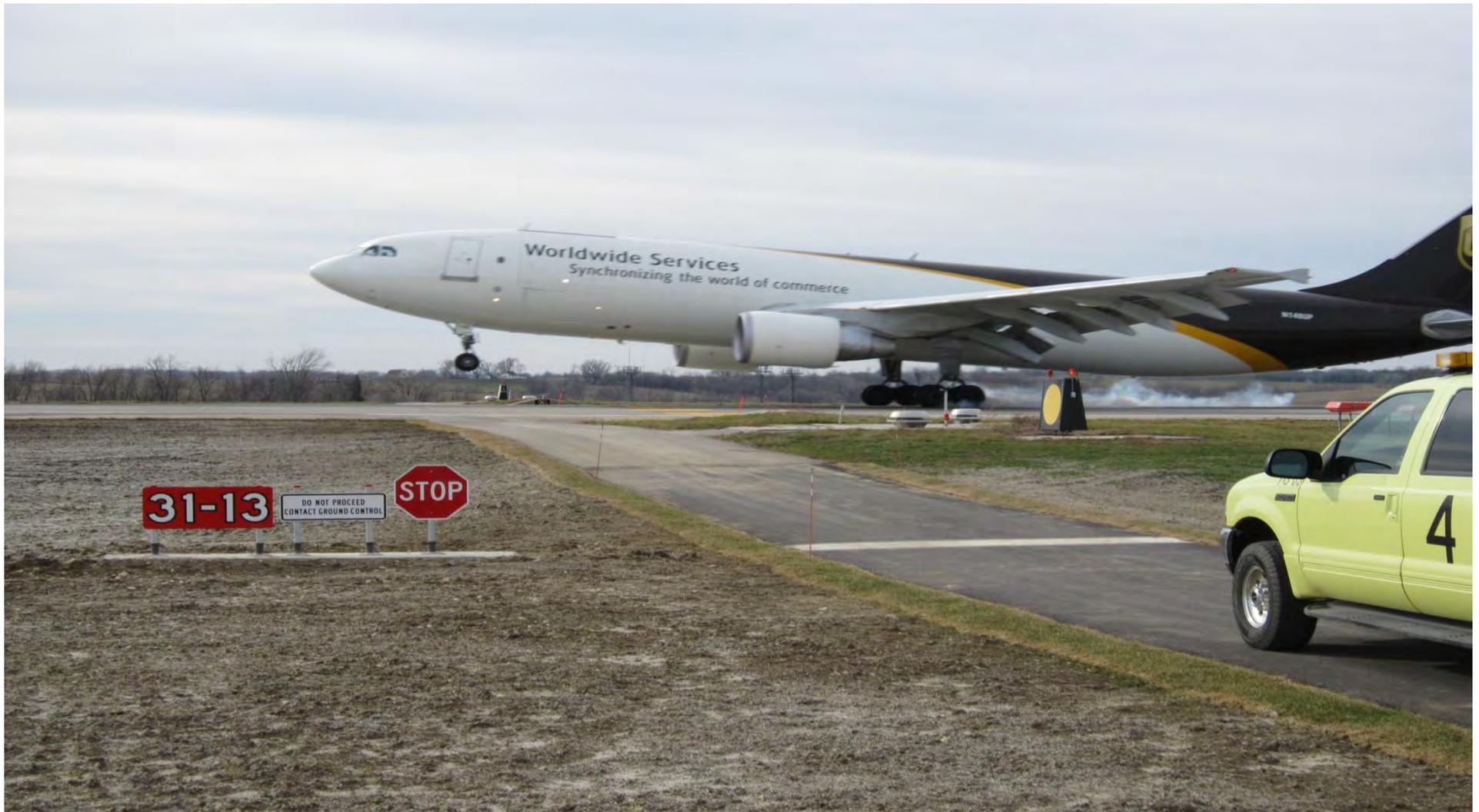
Service roads that enter runways should have vehicle roadway signs installed at the boundary of the runway safety area, in accordance with AC 150/5340-18F, Par 11, to help prevent inadvertent entry onto an active runway.
