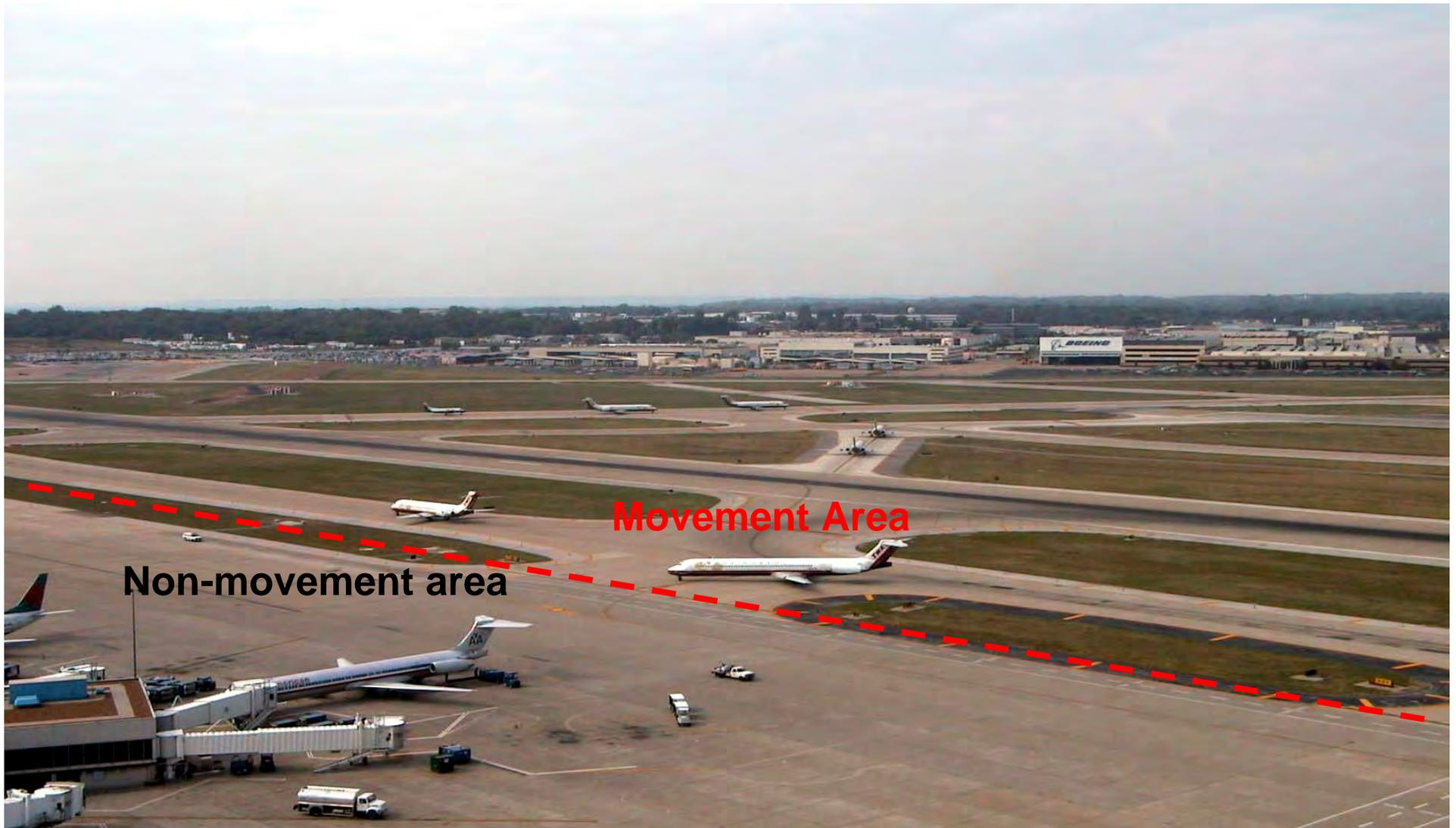
The **Movement Area** is the portion of the airfield where aircraft operate under the control of the Air Traffic Control Tower (ATCT). The movement area includes runways and taxiways. Normally, the apron area is non-movement area, however, at some airports, a taxiway may be located adjacent to the apron area and be under the control of Air Traffic Control.
