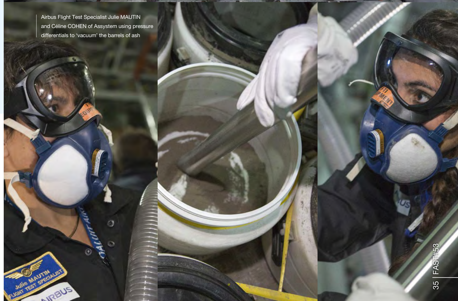
Inside the 'cavernous' A400M MSN 001 preparing for volcanic ash distribution
