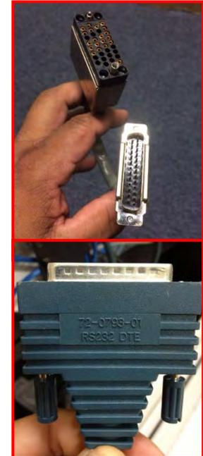
Required type should be **V.35 Cable Type**. Inspection of cable showed it to be **V.24 RS232 type** – not the correct connector.
