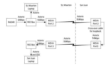
2.2.3 Please note that only one (1) channel of the MEVA satellite duplex circuit was used to transmit RADAR information from St. Maarten to San Juan. This indicates that the other channel of the duplex circuit could be used for returning a separate RADAR stream. This duplex operation exchanging separate RADAR streams was not tested and should be confirmed through further proof of concept testing before attempting to exchange RADAR data operationally.
