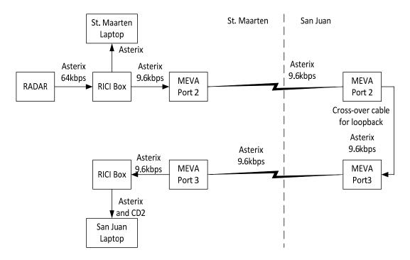
2.3 Only one (1) channel of the MEVA satellite duplex circuit was used to transmit RADAR information from Sint Maarten to San Juan. This indicates that the other channel of the duplex circuit could be used for returning a separate RADAR stream. This duplex operation exchanging separate RADAR streams was not tested and should be confirmed through futher proof of concept testing before attempting to exchange RADAR data operationally.
