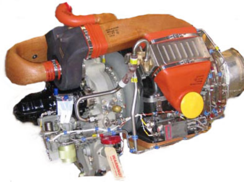
APU (Auxiliary Power Unit)
