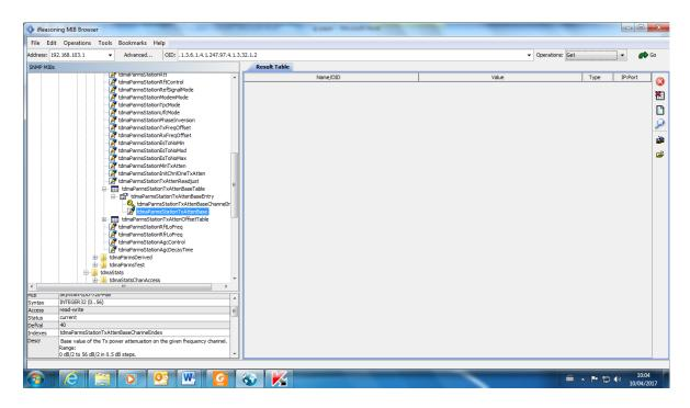
2.5 At the web page the parameter was 8 dB/2, here you have a local way to get it. When this parameter goes lo lows number that means that something is wrong with the transmission path. And we can with the get command have the same data locally. We did the same with demodulate channel input power:
