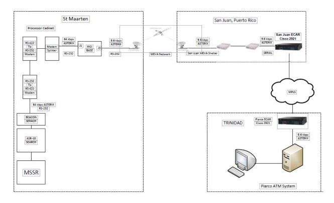
2.6.1 Please note that only one (1) channel of the MEVA satellite duplex circuit was used to transmit RADAR information from Sint Maarten to San Juan. The other channel of the duplex circuit will be used for a RADAR stream from Trinidad and Tobago to Sint Maarten. This duplex operation exchanging separate RADAR streams was not tested and should be confirmed through futher proof of concept testing before attempting to exchange RADAR data operationally.
