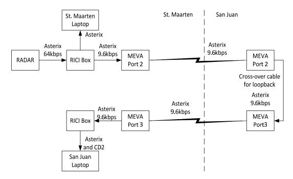
2.6 Further to the proof of concept tests, the following diagram depicts a possible solution to transmit RADAR data from Sint Maarten to Trinidad and Tobago over the MEVA/ECAR AFS Networks using one (1) RICI box in Sint Maarten over a serial connection:
