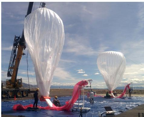
Project Loon balloons are capable of multi-day long-range flights at high altitudes, generally over FL600. Project Loon conducts a number of research flights launched and landed within the United States, as well as long range flights which often circumnavigate the globe.
