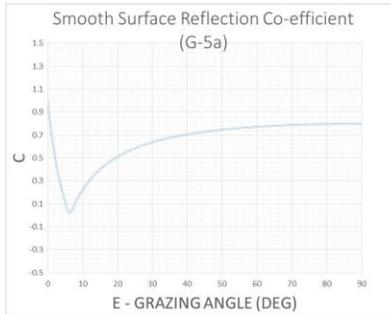
**Figure 2 – Fresnel Coefficient Plot for Smooth Surface**
