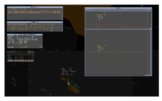
According to the destination airport and the landing runway a glide path cone is defined. The APM function generates a conflict if the position of an aircraft is in deviation (vertical or lateral) with respect to the nominal descending angle. The condition of deviation is calculated taking into account to different thresholds: one for lateral deviation and one for vertical deviation.
