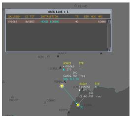
I4D capability to support the sharing of 4D trajectory between ground and air systems, the provision of time constraints at a specific point (e.g. during the descent/approach phase) and the monitoring of the aircraft behavior respect to the assigned constraint.
