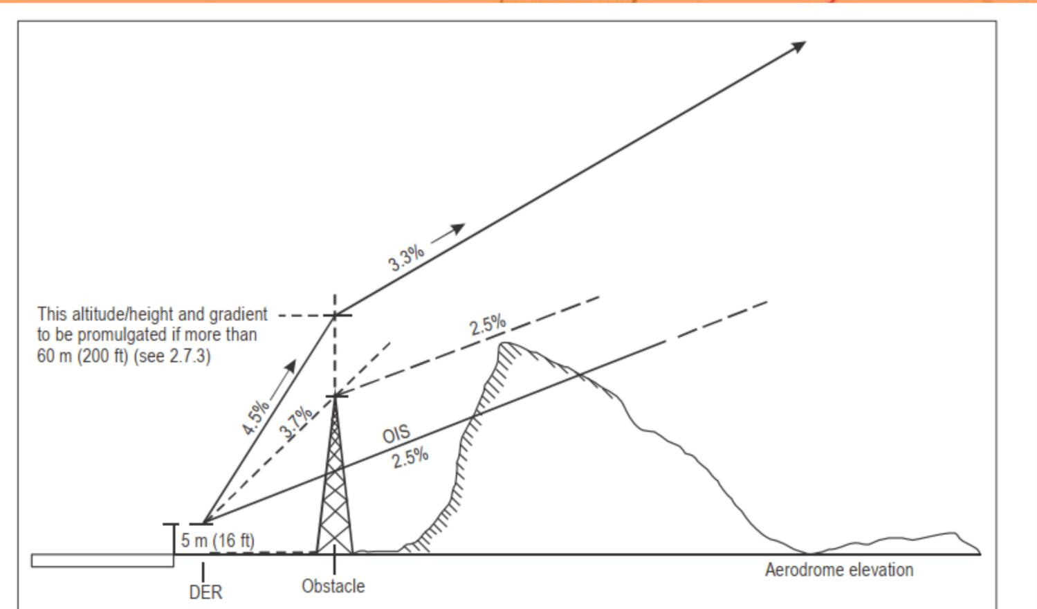
Figure I-3-2-2. Procedure design gradient
