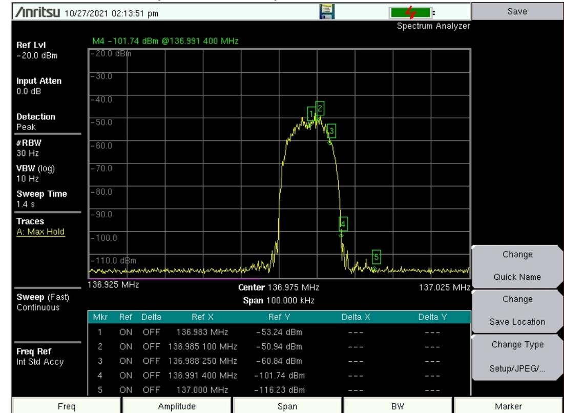
Out of Band (OoB) power at 137 MHz is attenuated higher than 60 dB from the In band AMS(R)S signal
