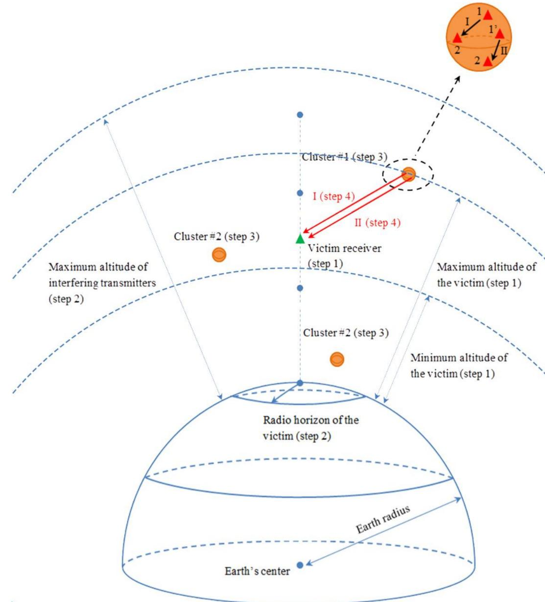
Figure adapted from WDT PDN Rep. ITU-R [NON-SAFETY AMS CHARACTERISTICS AND SHARING STUDIES]
