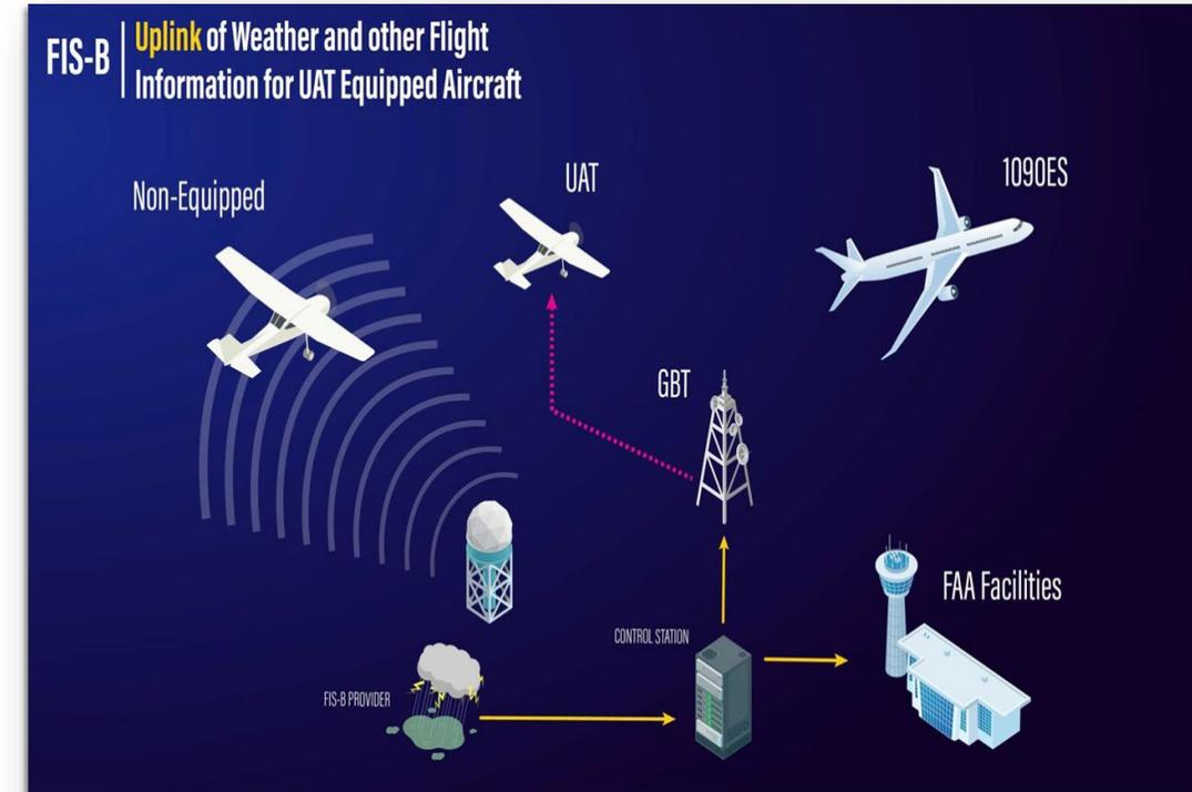
The **yellow arrows** show ground-based data flow from the Flight Planning systems to the control station, then the ground-based towers (GBT). The **pink arrows** show the transmitted data flow to UAT equipped aircraft.
