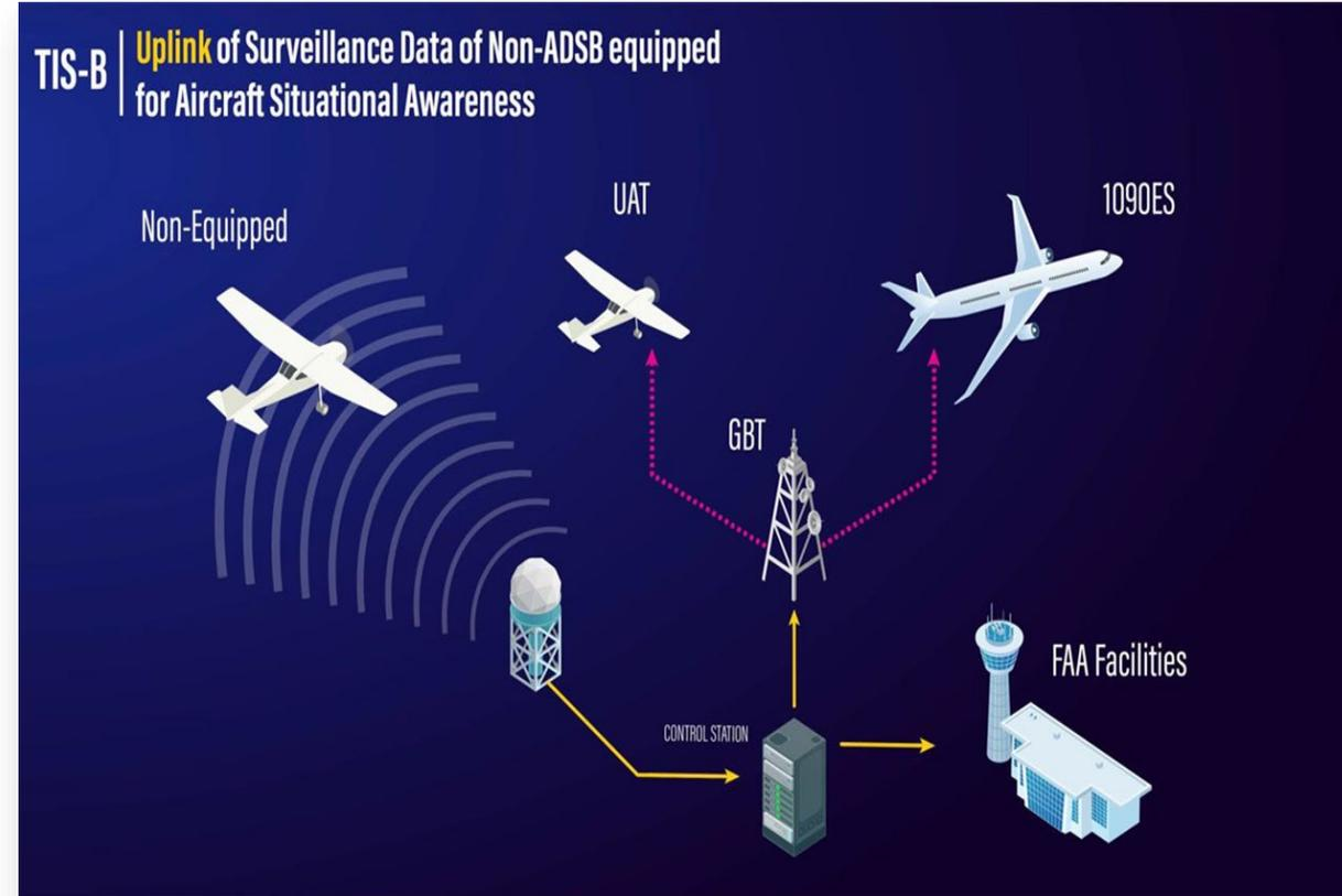
The **yellow arrows** show ground-based data flow from the receiver about non-ADS-B equipped aircraft to the control station, then the ground-based towers (GBT). The **pink arrows** show the transmitted data flow to ADS-B equipped aircraft.
