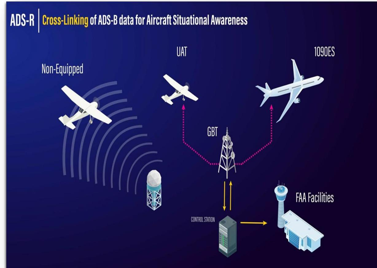
The **yellow arrows** show ground-based data flow from the receiver about non-ADS-B equipped aircraft to the control station, then the ground-based towers (GBT). The **pink arrows** show the transmitted data flow to ADS-B equipped aircraft.
