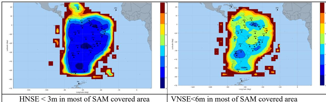
2.14 Measured position accuracy performances remain very efficient and fully compatible with APV-I vertical guidance approaches.
