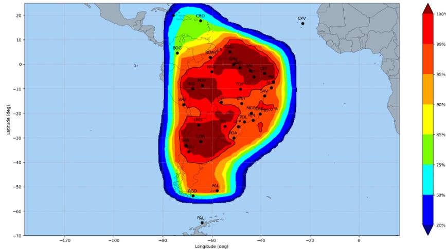
Figure 3: LPV / APV-I service level availability under very strong ionosphere conditions (selected day 2023-02-11)
