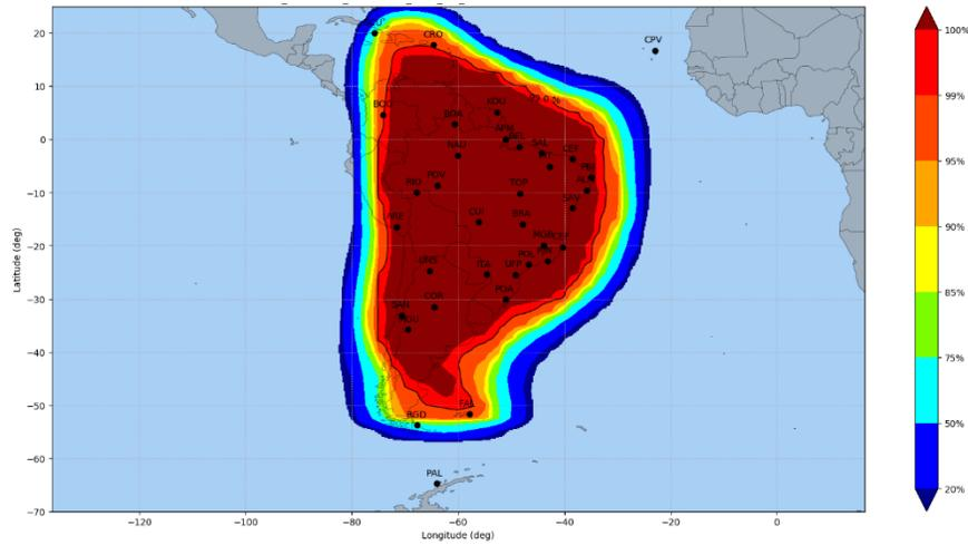
Figure 1 : LPV / APV-I service level availability under nominal ionosphere conditions (selected day 2021-08-16)
