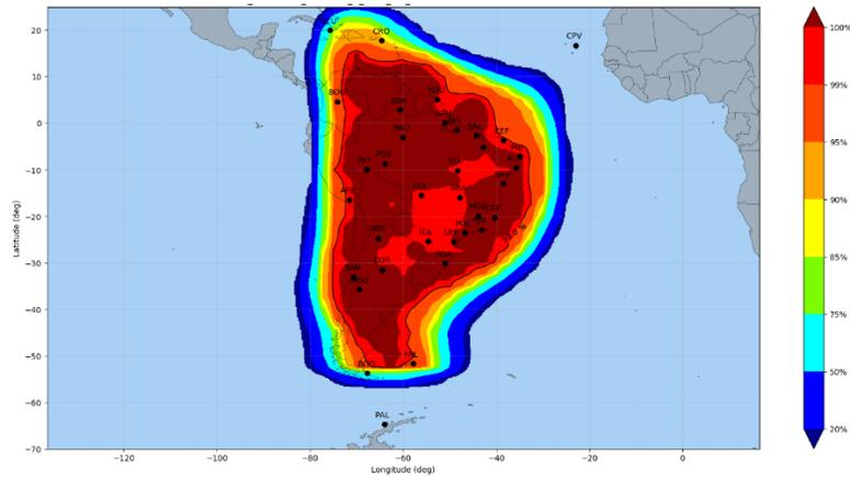
Figure 2: LPV / APV-I service level availability under active ionosphere conditions (selected day 2023-01-09)
