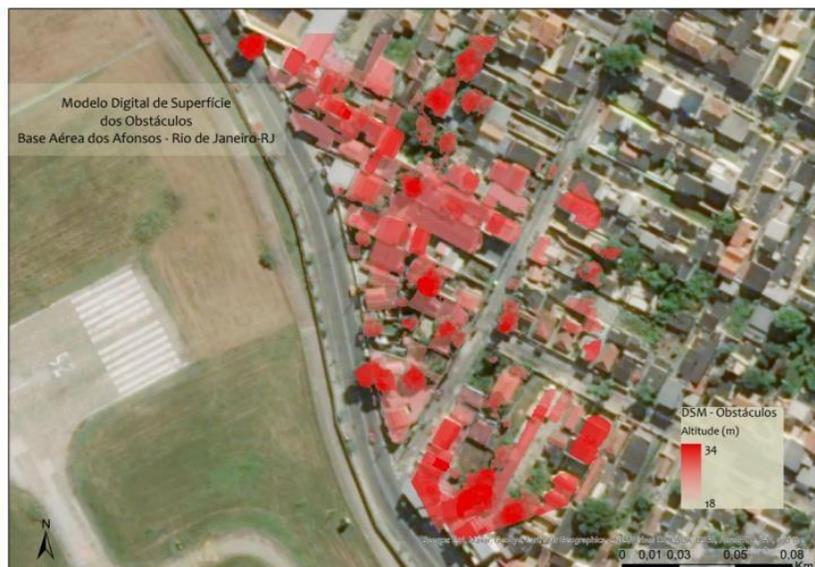
Figure 9: Digital surface model of obstacles located in the approach area of threshold 29 of the Campo Délio Jardim de Mattos (SBAF) aerodrome
