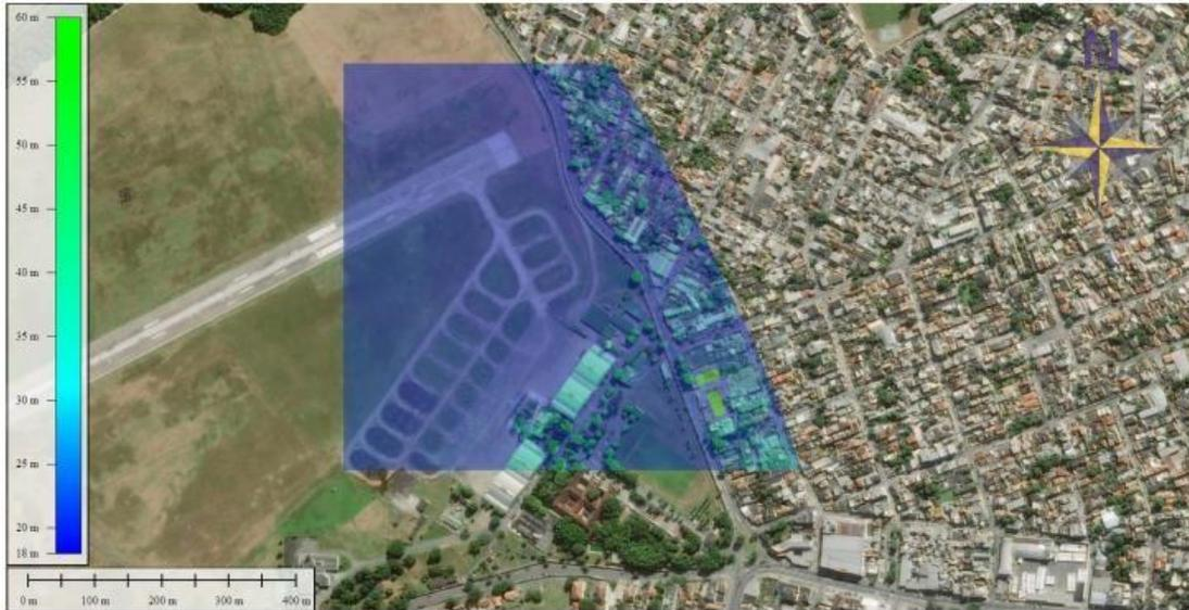
Figure 6: Map of the digital surface model close to the runway threshold
