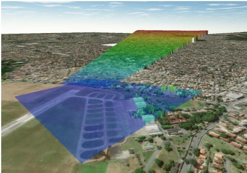
Figure 7: Digital surface model of buildings in the area of influence of the approach ramp and 3D takeoffs generated from the OLS and aerial survey with drone
