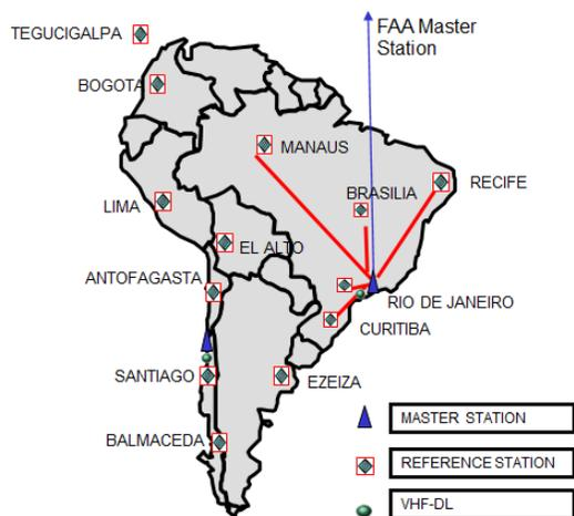
Figure 1 – Master and Reference Stations used in the SBAS test bed in 2002.
