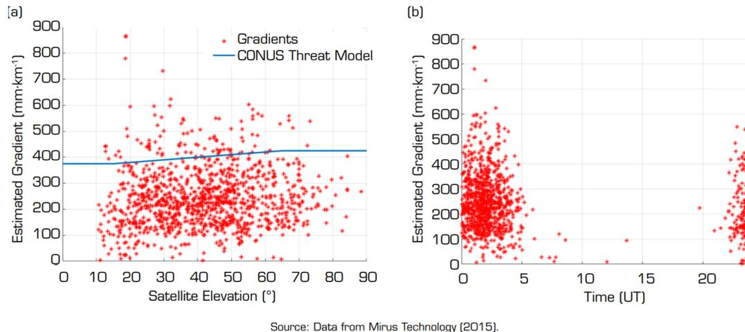
Figure 5 – Ionospheric gradients observed in Brazil. (a) Distribution based on the satellite elevation angle, CONUS threat model as reference; (b) Distribution based on UTC time
