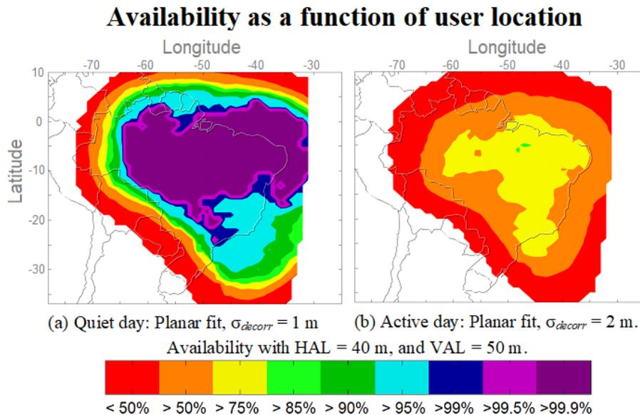
Figure 2 – Availability graphs obtained for days with high and low activity, using different parameters with planar fit interpolation, as presented in Marini-Pereira et al. (2021a).
