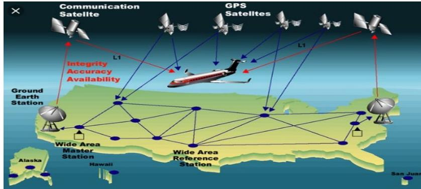
Figure 4 – Configuration of an SBAS service operation
