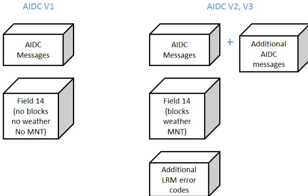
6.2.4.4 The diagram shows that AIDC messages supported in AIDC Version 1 is included in AIDC V2 and V3. As such, an AIDC V1 ATSU is interoperable with an AIDC V2 or 3 ATSU. The additional messages in AIDC V2 and V3 are not supported by AIDC V1. However, this could easily be controlled procedurally by simply not sending these messages.
