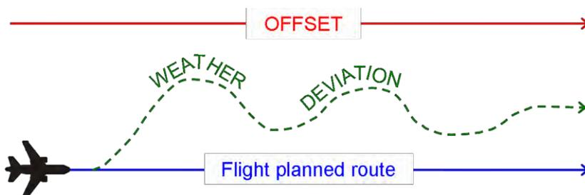
4.2.4.6.3 An offset is a flight trajectory that is parallel to the original route, offset by a specified distance and direction. Once an aircraft is established on the offset, separation may be applied solely based on the offset path.
