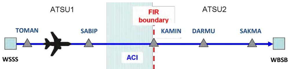
4.2.5.5 Field 15 information transmitted by ATSU1 to ATSU2 should commence at (or before) SABIP. This permits ATSU2 to calculate the profile of the aircraft commencing at the ACI boundary.
