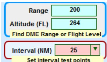
Note that in this example the field **Range** has been set to 200 NM (the program will find all DME stations within a range of 200 NM from each test point) and the field **Interval** to 25 NM (test points are separated by about 25 NM from each other). The number of found DME stations for each test point is presented in the list.
