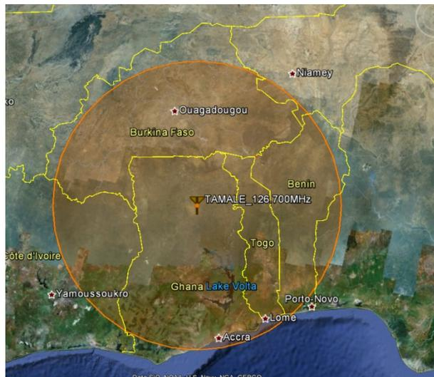
Note that in this case the coverage (which is also the protected coverage) for Tamale ACC extends to well outside the FIR ACCRA.
