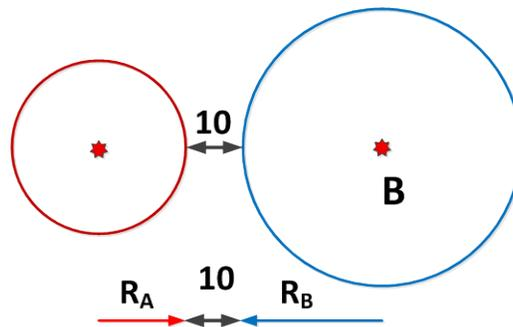
**Figure H-15 Minimum separation between circular facilities operating on adjacent frequencies**
