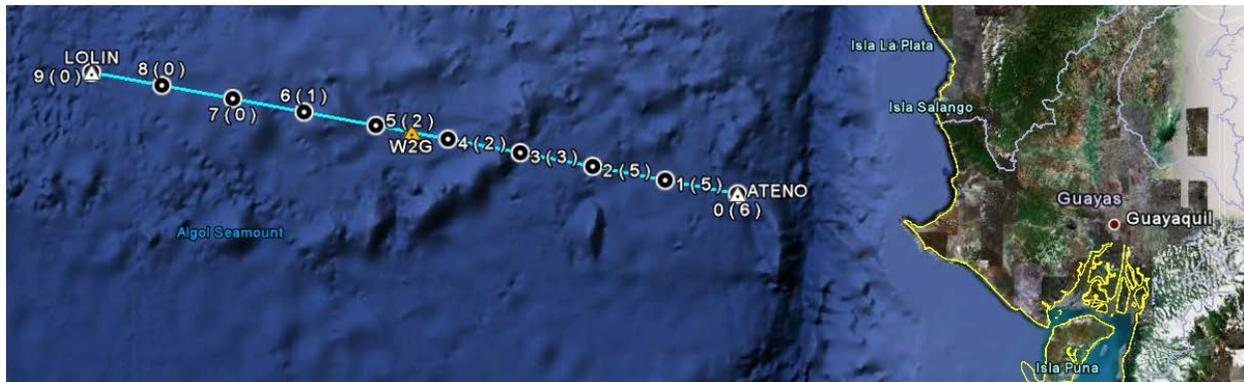
9.6.1.7 For each test point (including the start and end point) the number of the position of the test point (column **POS** in the table) is plotted with the test point. The number in between brackets represents the number of found DME within “range of this test point. In this example, the “range” was set to 200 NM; the interval to 25 NM.
