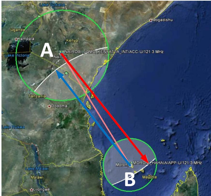
Figure H-6 Interference between two facilities with a circular DOC as presented with Frequency Finder
