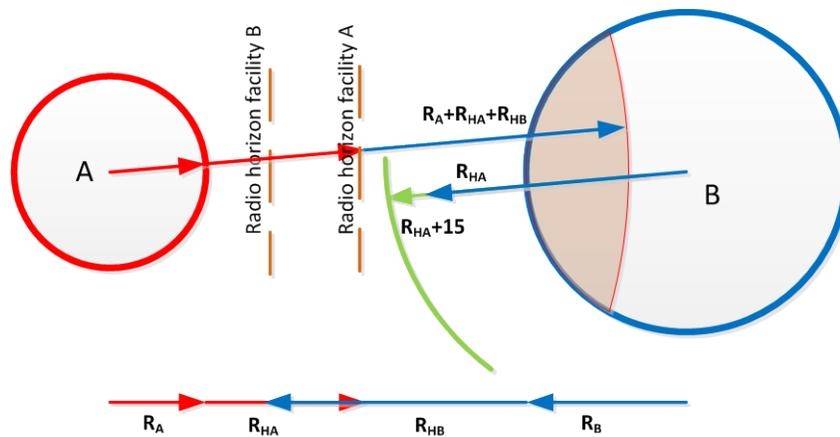
Figure H-13 Interference mechanism between broadcast services; interference contours
