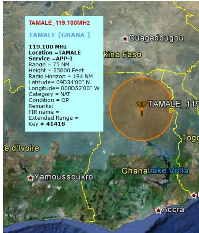
When clicking on the icon for Tamale on the map, Google Earth will display a balloon containing data which is pertinent to the frequency assignment. For the presentation of the coverage on the map with Google Earth, the location icon and the circles or polygons describing the coverage (DOC – Range) are both orange.
