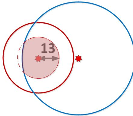
**Figure H-19 Interference contour/area when the minimum separation distance requirements between broadcast services operating on adjacent frequencies are not satisfied.**
