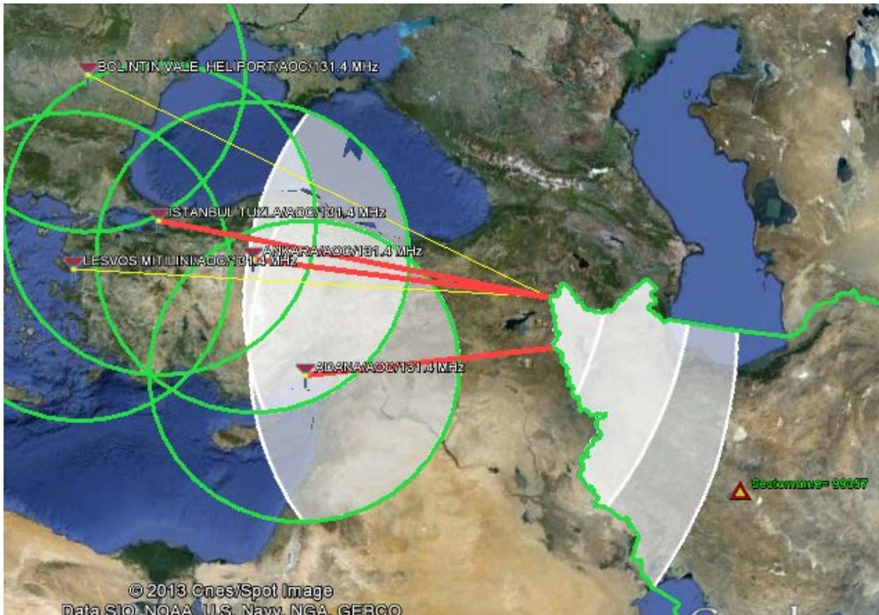
Co-frequency assignments that are incompatible are connected to the frequency being tested (FIR Tehran in the above figure) along the shortest path and connected with a red line. In addition, Frequency Finder calculates the area in which interference may be expected and presents this with a white shaded background on the map. Frequency assignments that are compatible are connected to the frequency being tested with a yellow line.
