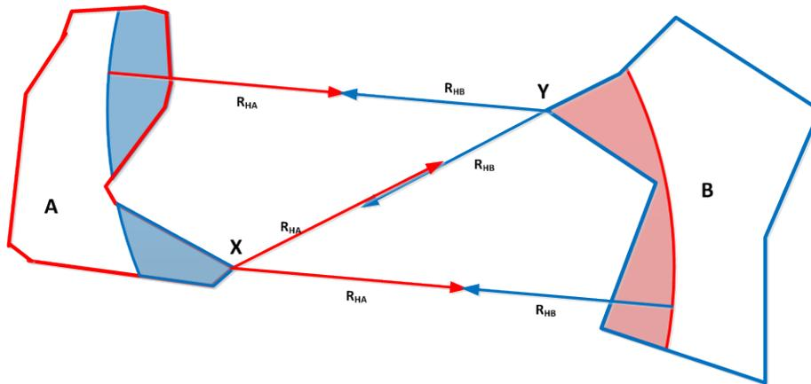
Figure H-9 Interference contours for two area services
