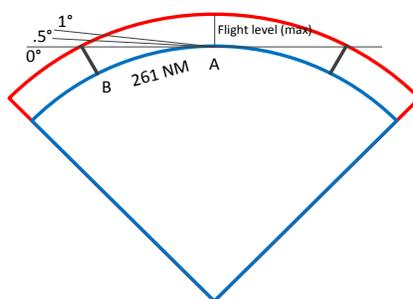
**Figure B-1 Reduction in distance to the transmitter when receiving above the horizontal plane through the ground antenna**
