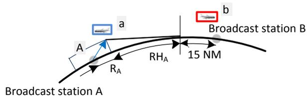
Figure H-11 Interference mechanism between broadcast services
