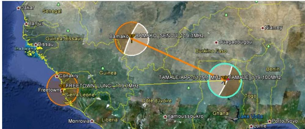
Co-frequency interference between Tamale and Bamako-Senou in the AFI Region; both coverage areas are partially being interfered by each other (white circle segment)
