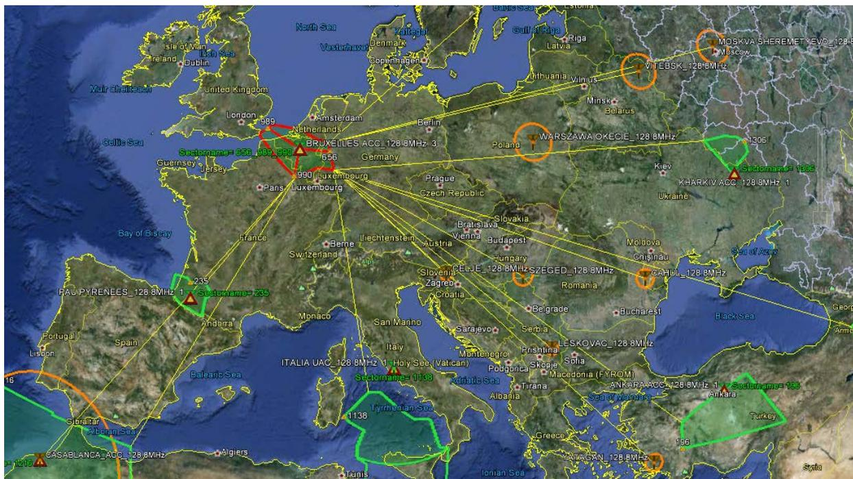
2. Co-frequency interference (frequency assignments are not compatible)
