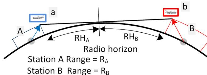
**Figure H-3 Separation based on radio line-of-sight**
