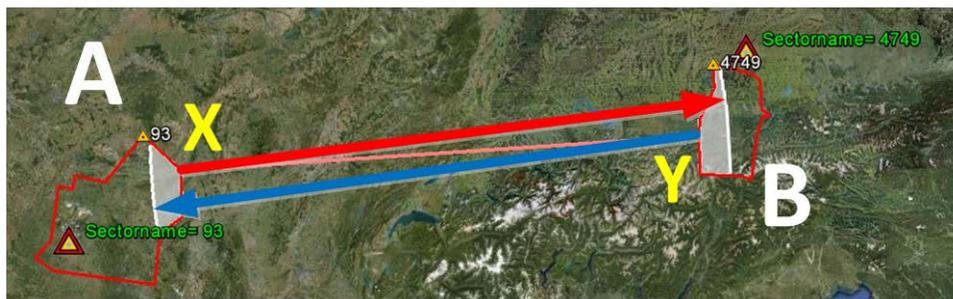
Figure H-10 Interference contours for two area services as is presented with Frequency Finder
