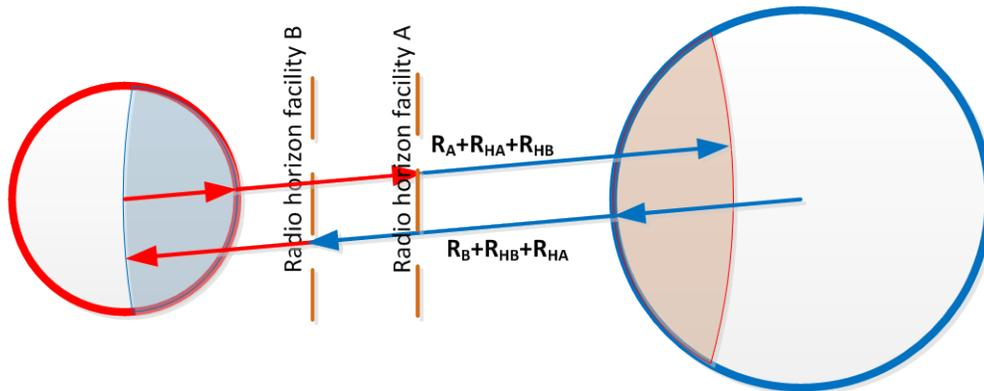
**Figure H-5 Interference contours for two circular services**
