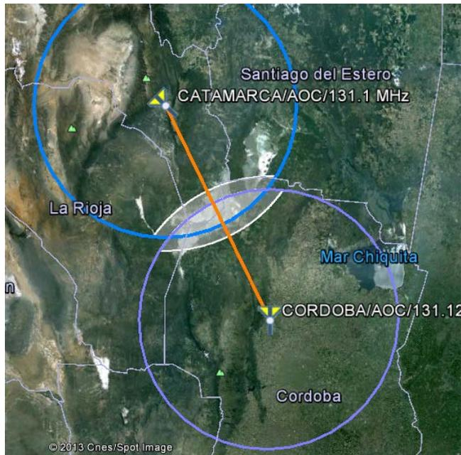
Adjacent frequency interference shows as a circle-segment with a buffer zone of 10 NM outside the coverage of the interferer.
