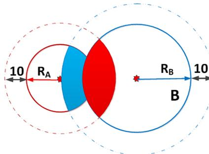
**Figure H-16 Interference contours/areas between circular facilities operating on adjacent frequencies**
