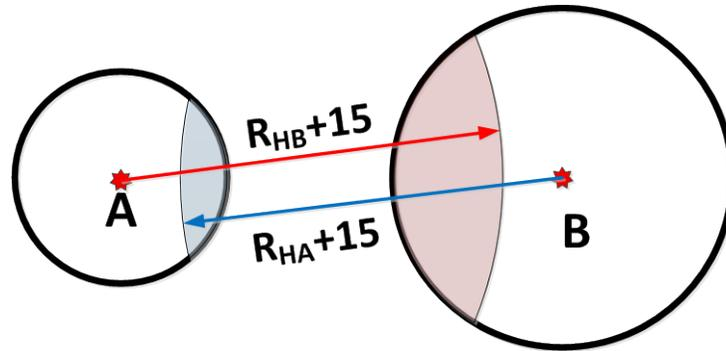
Figure H-11 Interference mechanism between broadcast services
