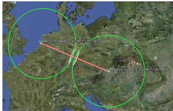
Figure H-12 Interference mechanism between circular broadcast services as presented with Frequency Finder
