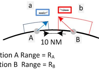
**Figure H-14 Adjacent frequency separation for air-ground services**
