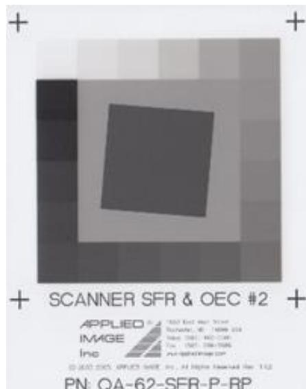
**Figure D.4 — Test pattern: ISO 16067-1. Note that the physical distance between the fiducials on the standardized test pattern is 66.8 mm.**
