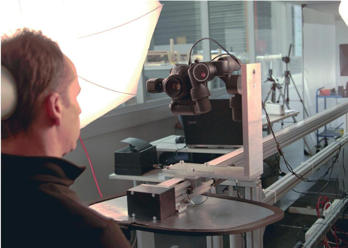
**Figure F.2 – Bench created to rapidly capture a number of pictures at different distances**
