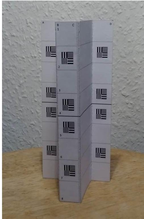
**Figure B.2 — Ready to use simple magnification distortion target. One can see the millimetre markers on the nose level, and the markers in 2 cm distance on nose and eye level as well as the resolution targets with one and two line pairs per millimetre.**
