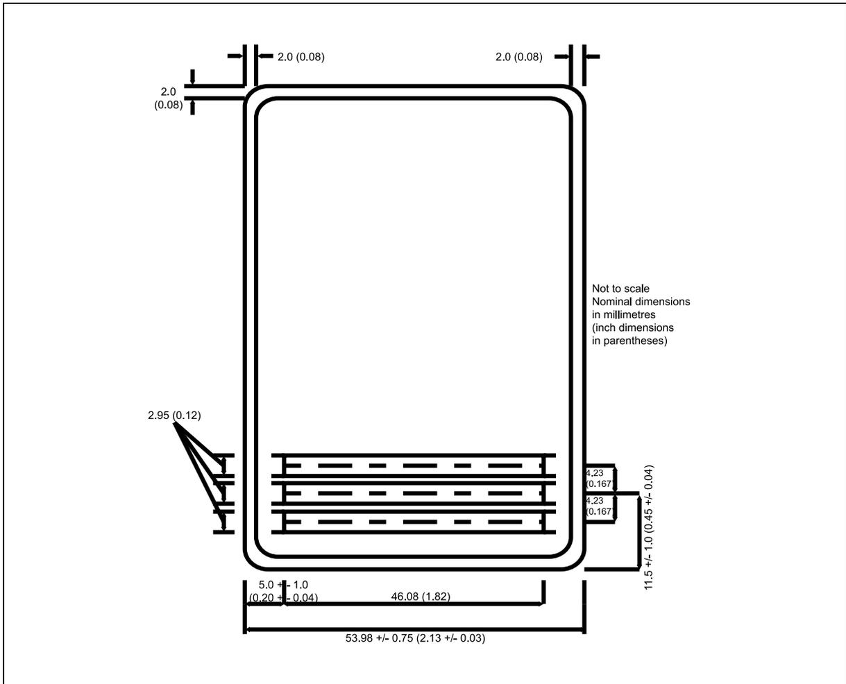
Figure 21: Additional specification for CAN placement in portrait-oriented TD1-size documents
