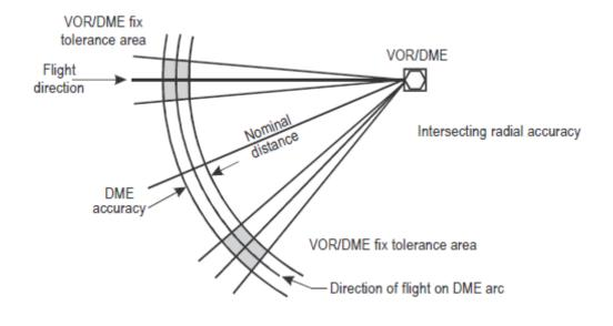
Figure I-2-2-1. Intersection fix tolerance areas
