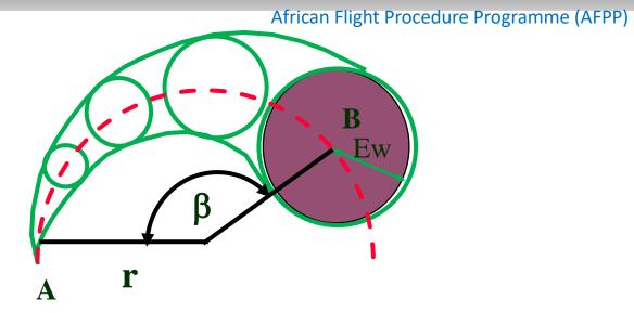
W: Wind speed (in m/s) and T: Time in s Ew is the wind effect (radius of circle in m with  $T(AB) = (\beta r) / TAS$  $\beta$  In rd, r in m, TAS in m/s
