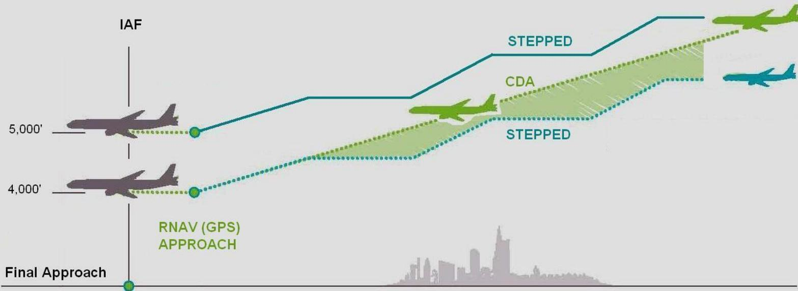
STAR altitude windows and procedure height constraints should be designed **to allow most aircraft to descend unimpeded.**
