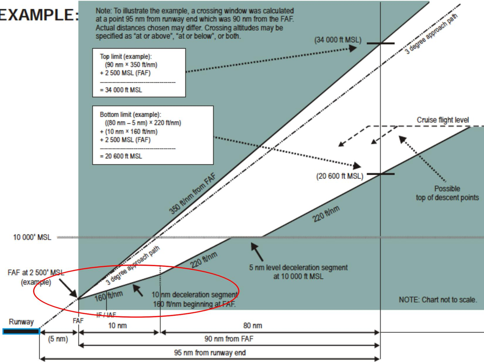
This example shows a STAR linked to an **instrument approach** in an optimized CDO procedure and should allow most FMSs to perform fully automated lateral navigation/vertical navigation (LNAV/VNAV) descent.
