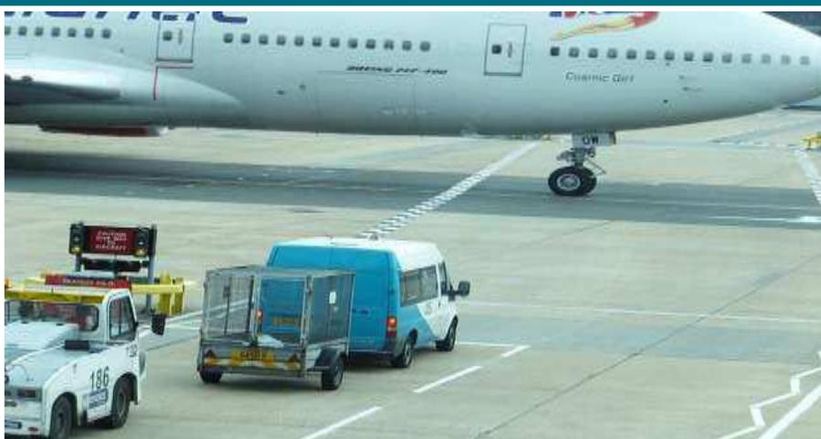
UNCONTROLLED VEHICLE CROSSING OF LIVE TAXIWAY WITH GOOD USE OF SURFACE MARKINGS (HOLD/STOP & ZIPPER), SIGNAGE AND WARNING LIGHTS
