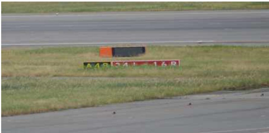
**ENHANCED VARIABLE MESSAGE SIGNAGE AT RUNWAY HOLDING POINT TRIALLED BY JAPANESE CAA AT TOKYO NARITA TO STRENGTHEN EXISTING RUNWAY INCURSION PREVENTION MEASURES – SIGN SHOWING BLANK**
