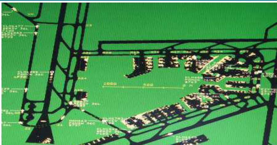
GROUND MOVEMENT RADAR – USED BY ATC AS PART OF ASMGCR TO MONITOR NOT ONLY AIRCRAFT ON THE GROUND, BUT ALSO OPERATIONAL VEHICLES
