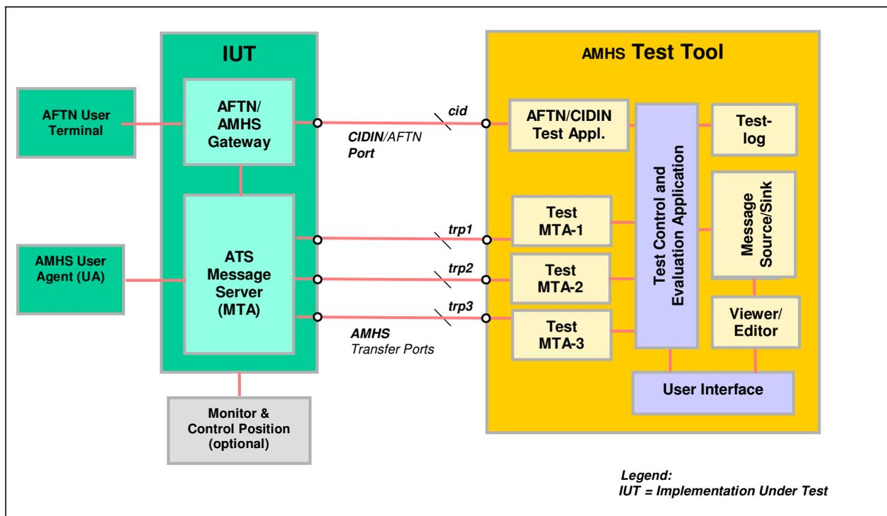
*Figure 1: AMHS Conformance Test Environment*
