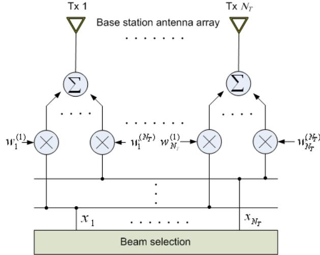
A linear array of  $N_T$  isotropic antenna elements with uniform spacing is considered. The data signals  $x_k$ ,  $k=1, \dots, N_T$  from the beam selector are directly multiplied by a set of weights  $U = \{\mathbf{w}_1, \mathbf{w}_2, \dots, \mathbf{w}_{N_T}\}$  to form a null at known DOE.  $\mathbf{w}_m = [w_1^{(m)}, w_2^{(m)}, \dots, w_{N_T}^{(m)}]$  is the  $m$ -th weight vector in row vector and is given by the following set of equations:
