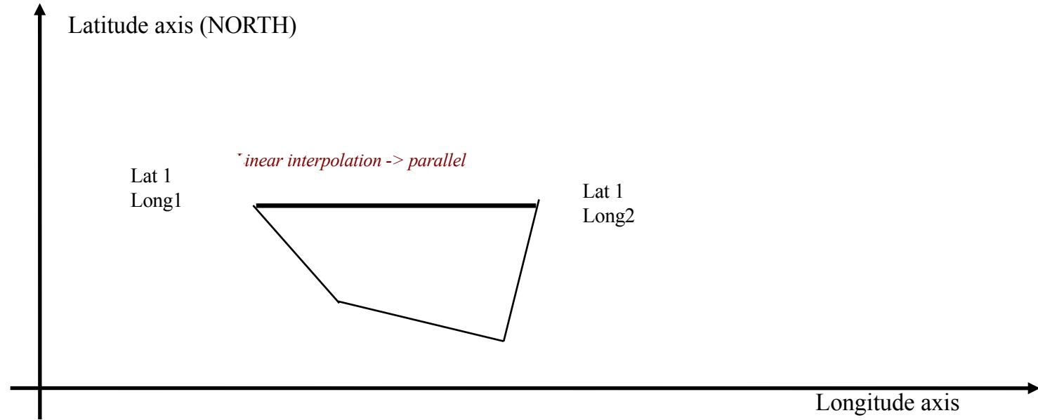
Linear interpolation in a conformal projection, e.g. Mercator
