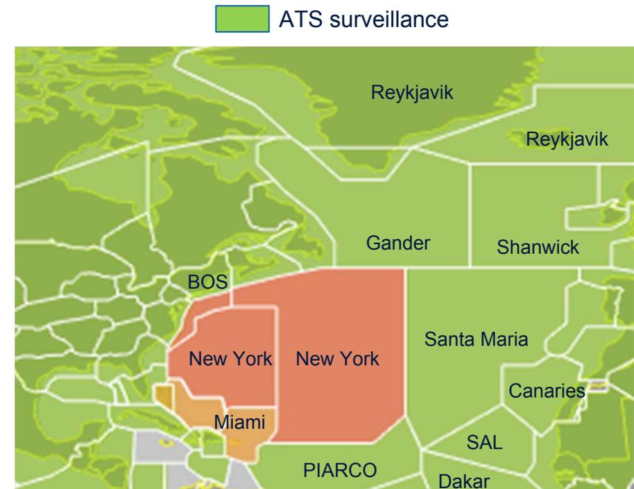
The NAT ANSPs are planning to implement 15 nm separation in 2018 using space-based ADS-B enabling significant improvements in operations
