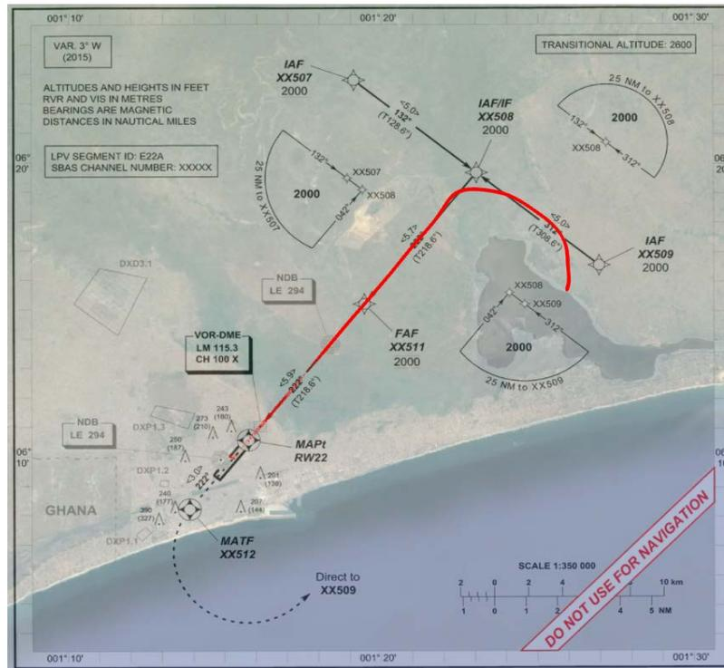
Figure 10: Recorded flight path vs. procedure chart
