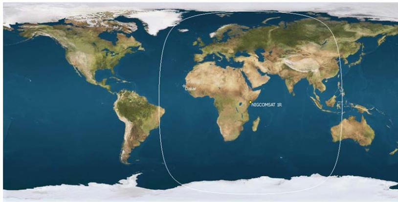
**Figure 5: NigComSat-1R coverage area**
