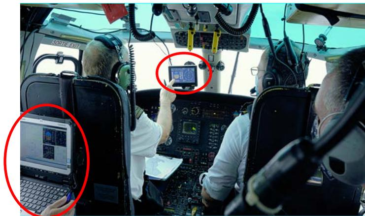
**Figure 12: Flight deck with external navigation display for SBAS demo flight**
