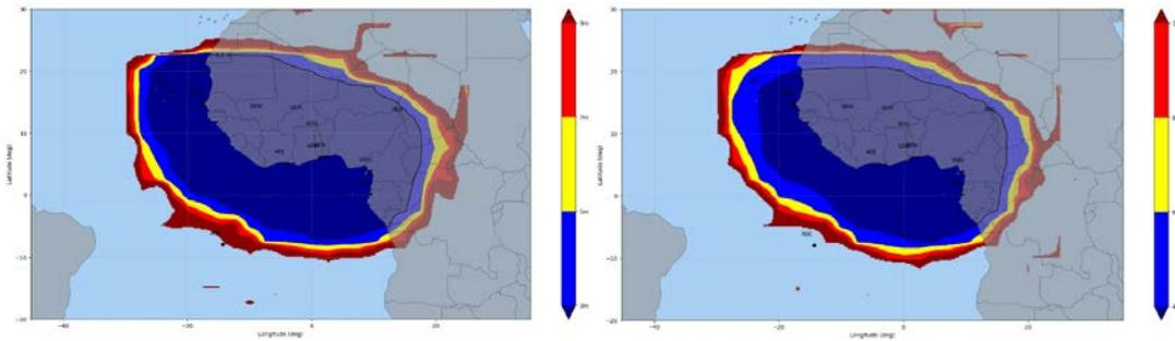
Figure 7: OS service availability (left: horizontal accuracy 3m@100%, right: vertical accuracy 4m@100%)
