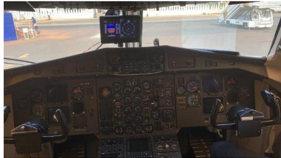
**Figure 9: Flight deck equipped with navigation display for SBAS demo flight**
