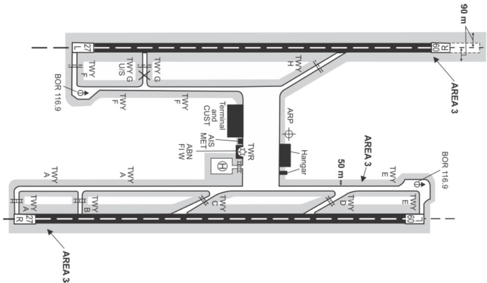
**Figure 5:** Terrain and obstacle data collection surface — Area 3
