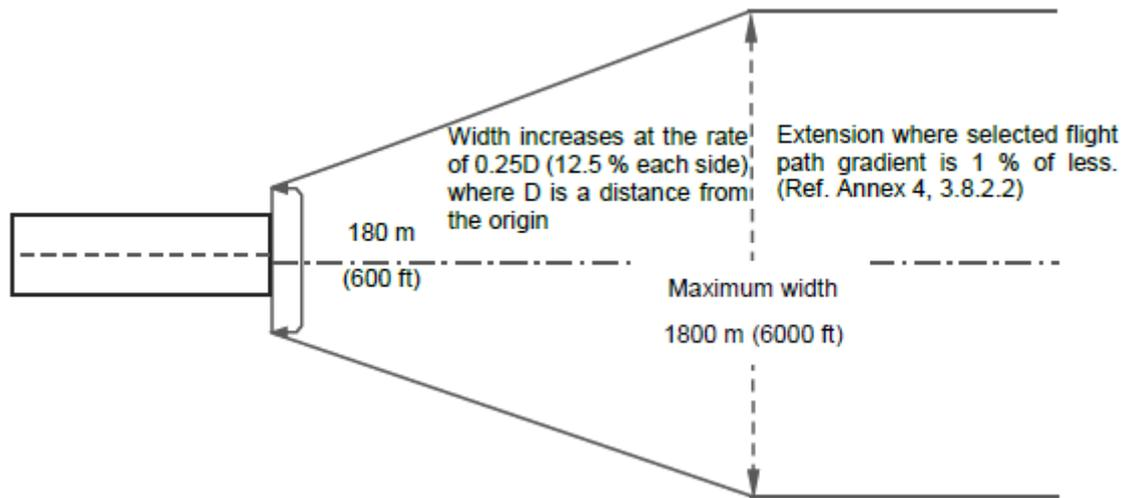
**Figure 8:** Graphical representation of take-off flight path area as defined in ICAO Annex 4
