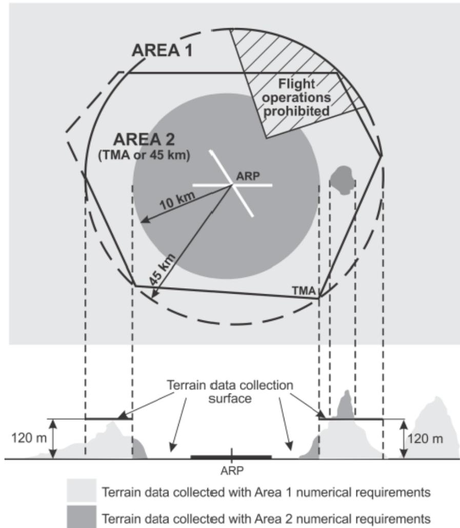
**Figure 3:** Terrain data collection surfaces — Area 1 and Area 2
