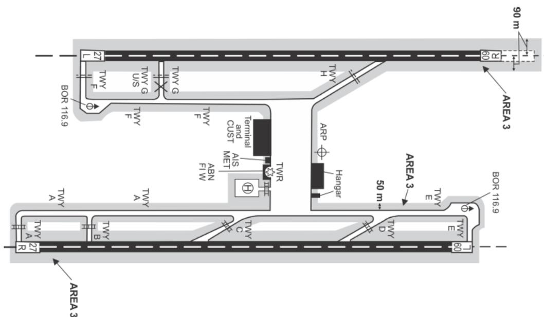
**Figure 12:** Obstacle data collection surface — Area 3
