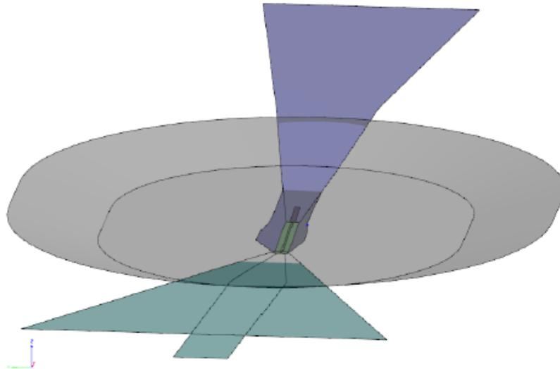
**Figure 1:** Graphical representation of the listed obstacle limitation surfaces
