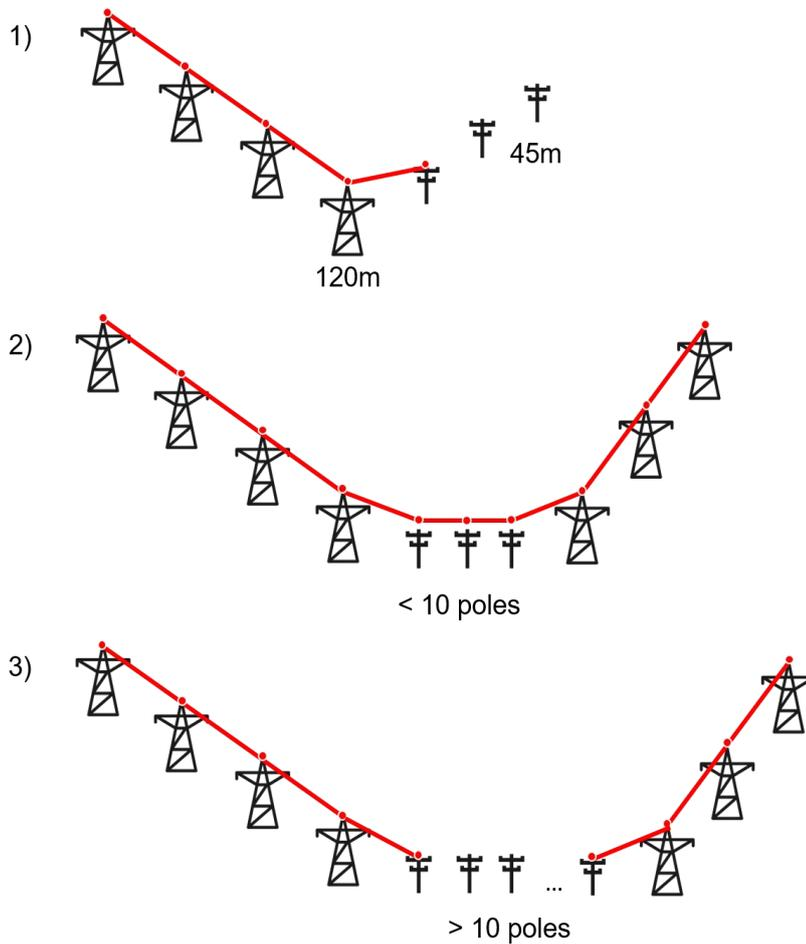
Figure A11: Capture of power lines with segments below the collection surface
