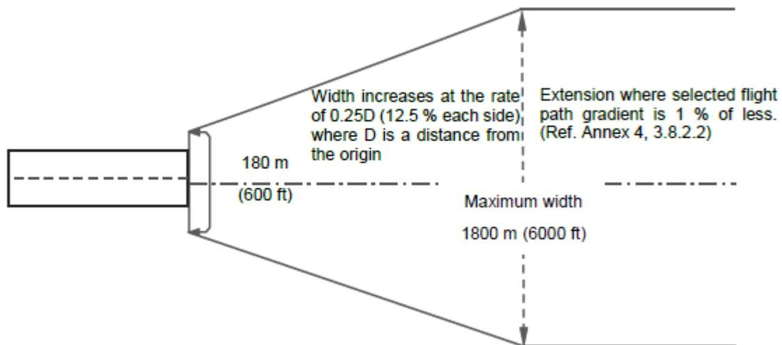
**Figure 2:** Graphical representation of take-off flight path area as defined in ICAO Annex 4
