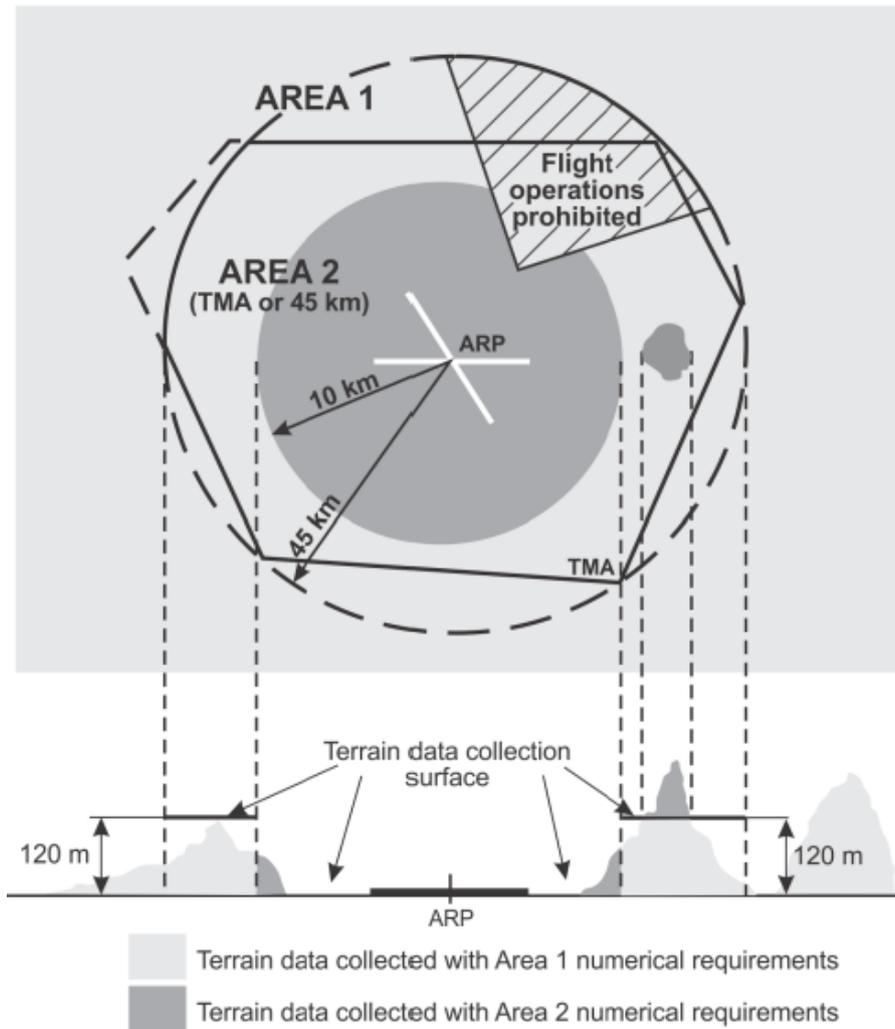
**Figure 5:** Terrain data collection surfaces — Area 1 and Area 2
