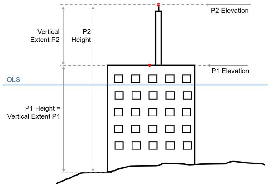
Figure A14: Example of a segmented obstacle
