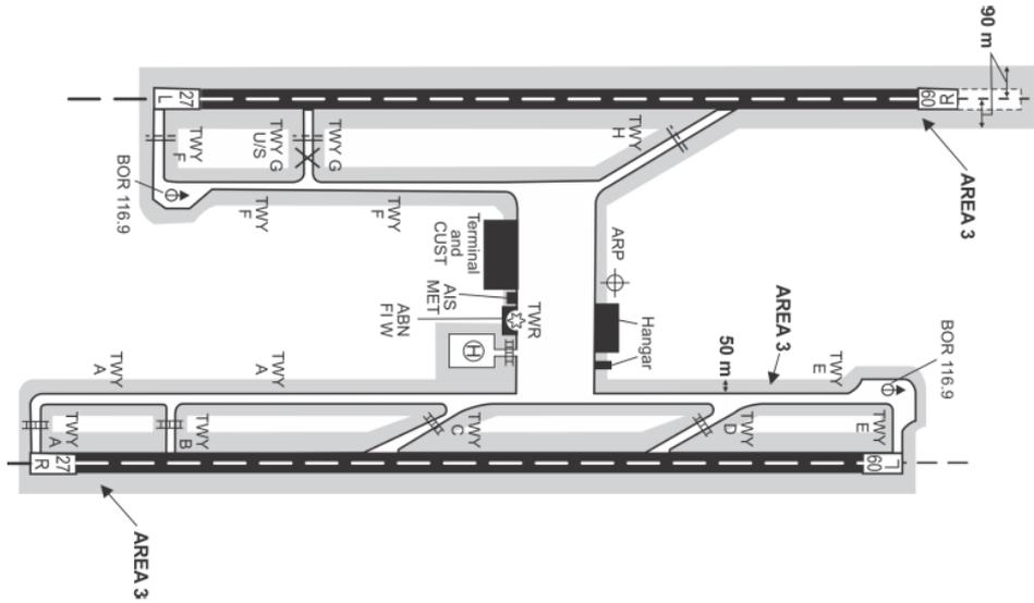
Figure 6: Terrain data collection surface — Area 3
