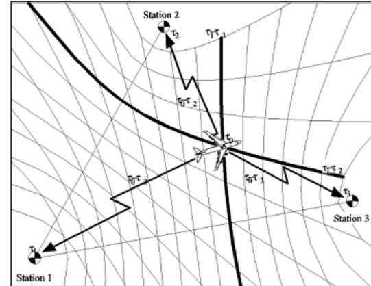
This principle can be extended to measure 3D positions : a 4<sup>th</sup> ground station is then required
