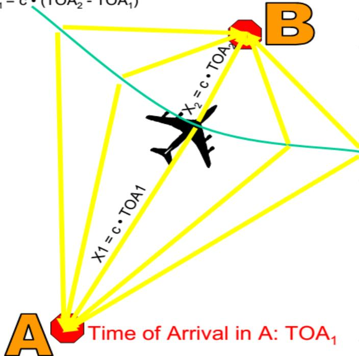
At a given time, the Aircraft is on the locus of points having the distance  $X_2 - X_1$  constant:
