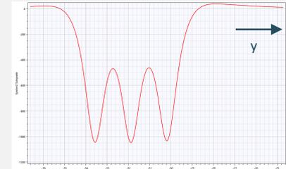
Example of longitudinal strain profile  $\epsilon_z(x, y)$
