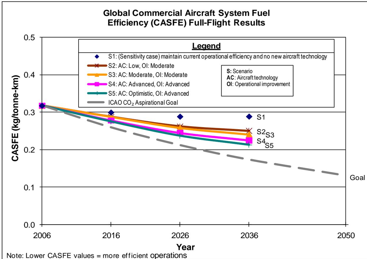
**Figure 6. Commercial Aircraft System Fuel Efficiency (CASFE) Full-Flight Results.**
