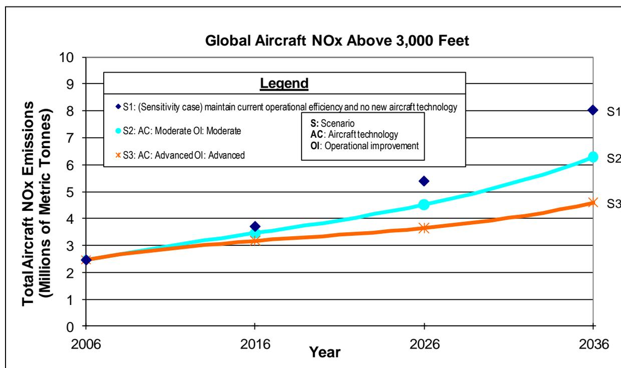
Figure 3. Total Global Aircraft NO<sub>x</sub> Above 3,000 Feet AGL.
