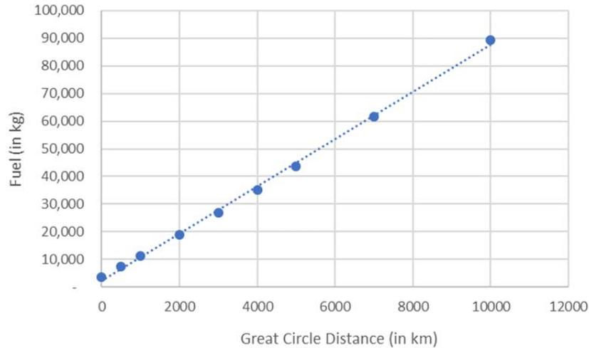
**Figure 11: Illustration of generic aircraft CEM**
