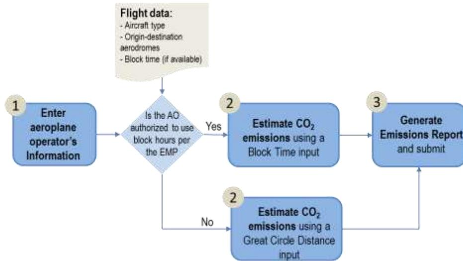
**Figure 12: Overview of the high-level functions of the potential CORSIA CO<sub>2</sub> Estimation and Reporting Tool**
