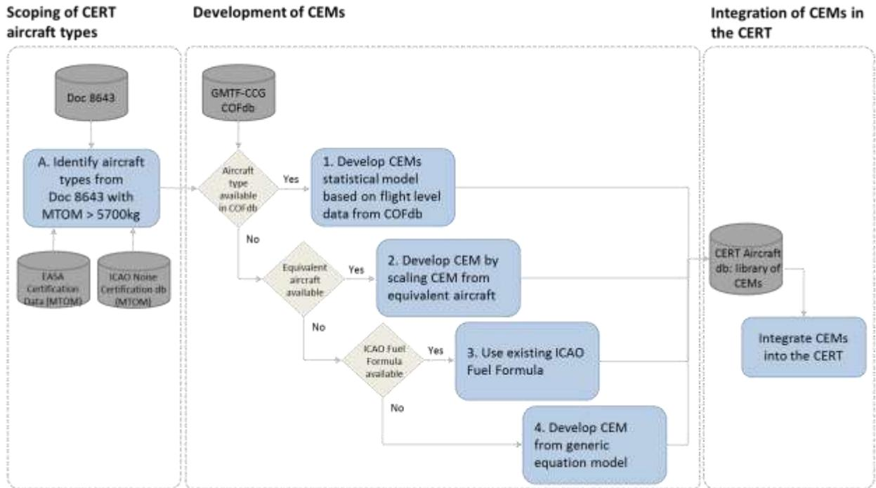
Figure 13: Summary of process for developing ICAO CO<sub>2</sub> Emissions Estimation Models (CEMs)
