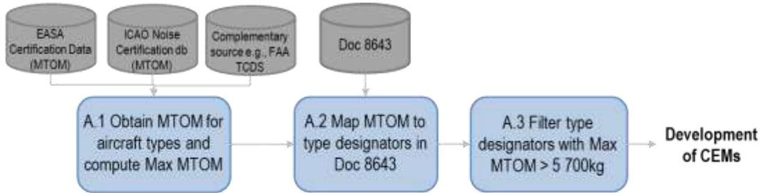
Doc 8643 has total of 10 020 aircraft types categorized as Amphibian, Helicopter, Landplane, SeaPlane or Tilt-wing. Further, each aircraft type has the manufacturer's name, ICAO Designator, engine type, engine count and wake turbulence category (WTC).
