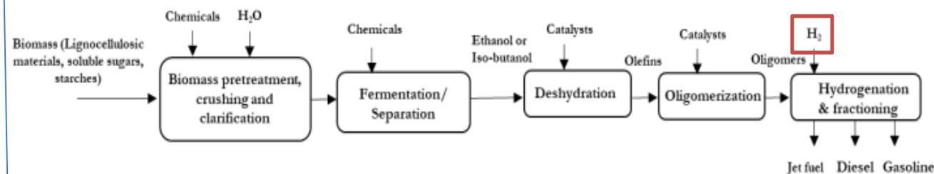
Figure 6: General process flow alcohol-to-jet pathway
