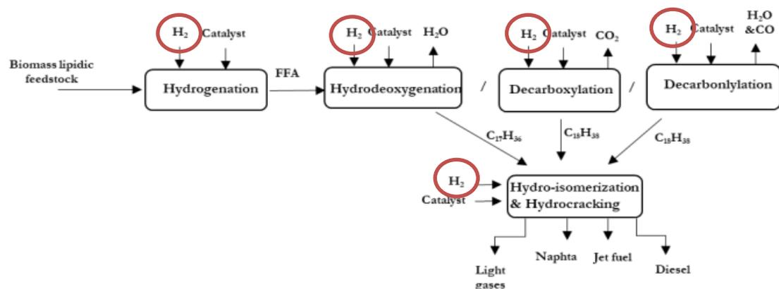
For ATJ, Hydrogen is also needed as a process input
