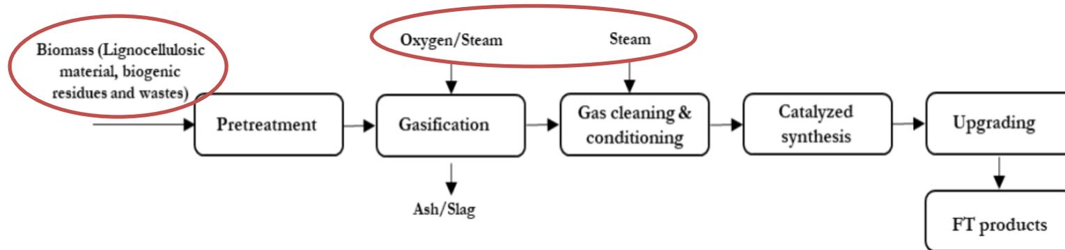
Figure 2: General process flow Fischer-Tropsch pathway
