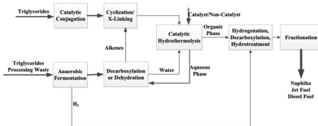
**Figure 224.** CHJ SAF conversion process from vegetable oils
