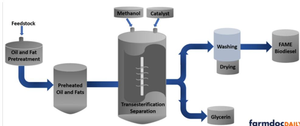
**Figure 246.** FAME biodiesel production process
