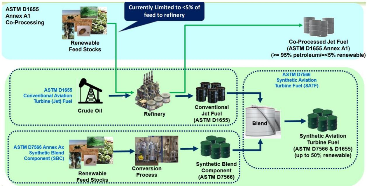
Figure 280. SAF co-processing process
