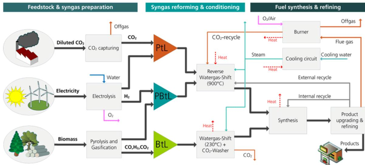
**Figure 235.** PtL SAF conversion process from carbon dioxide and biomass
