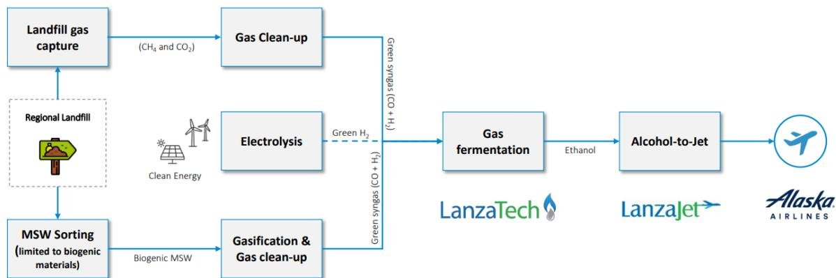
Figure 824. ATJ SAF Process From MSW Feedstock
