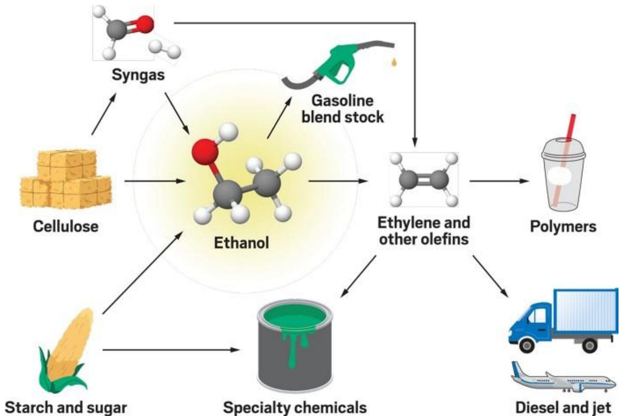
**Figure 802.** Ethanol as an intermediate to make fuels and chemicals from biomass
