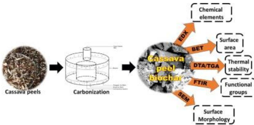
**Figure 413.** Biochar Production from Cassava Peels
