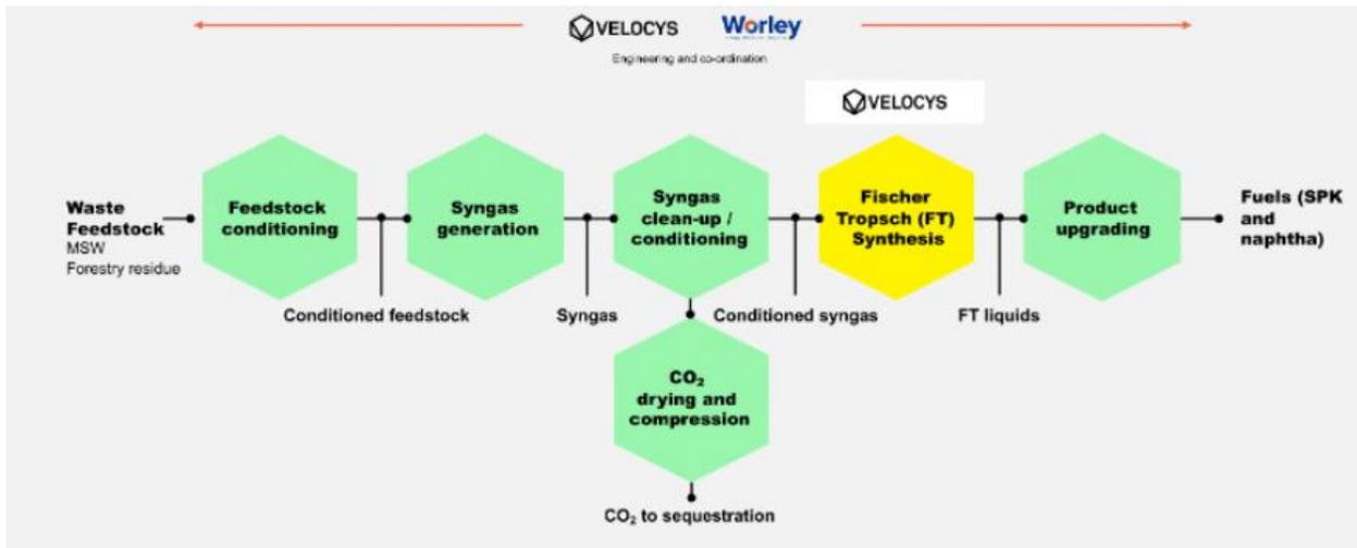
**Figure 835.** FT SAF process from MSW and forestry waste
