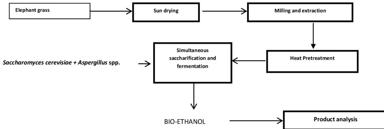
**Figure 58.** Process to make bioethanol from elephant grass
