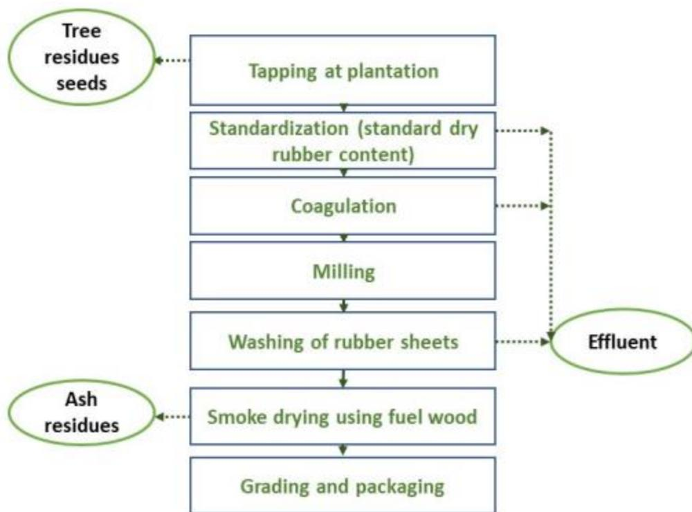
**Figure 613.** Rubber production process
