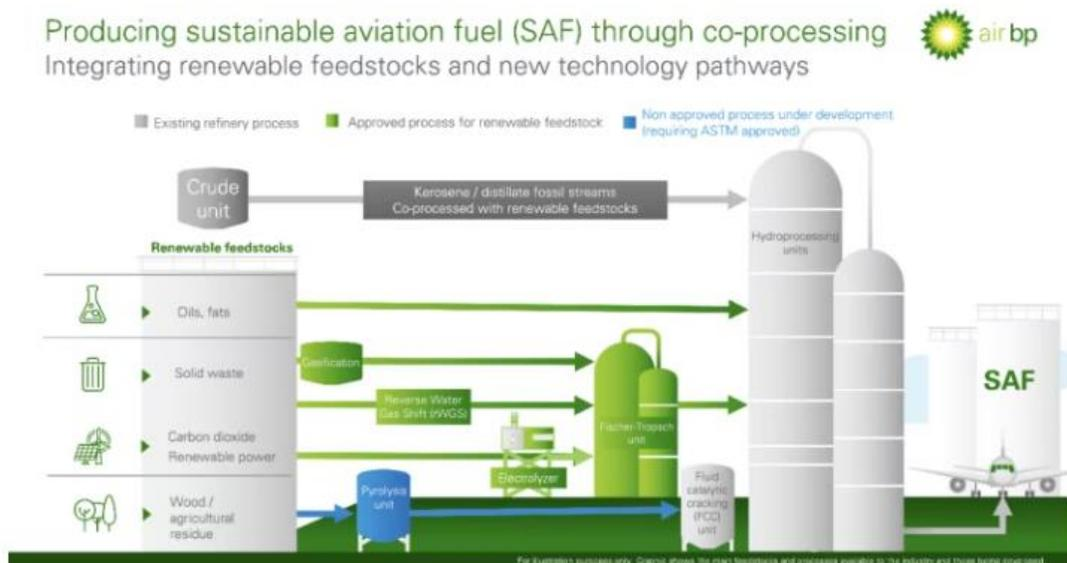
**Figure 29.** Co-processing pathways using various renewable feedstocks.
