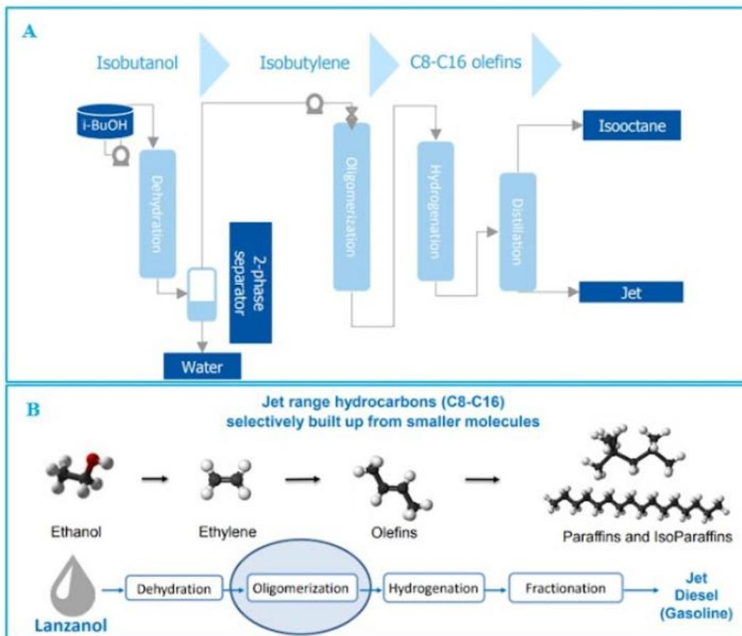
**Figure 568.** Process to convert bioethanol into SAF
