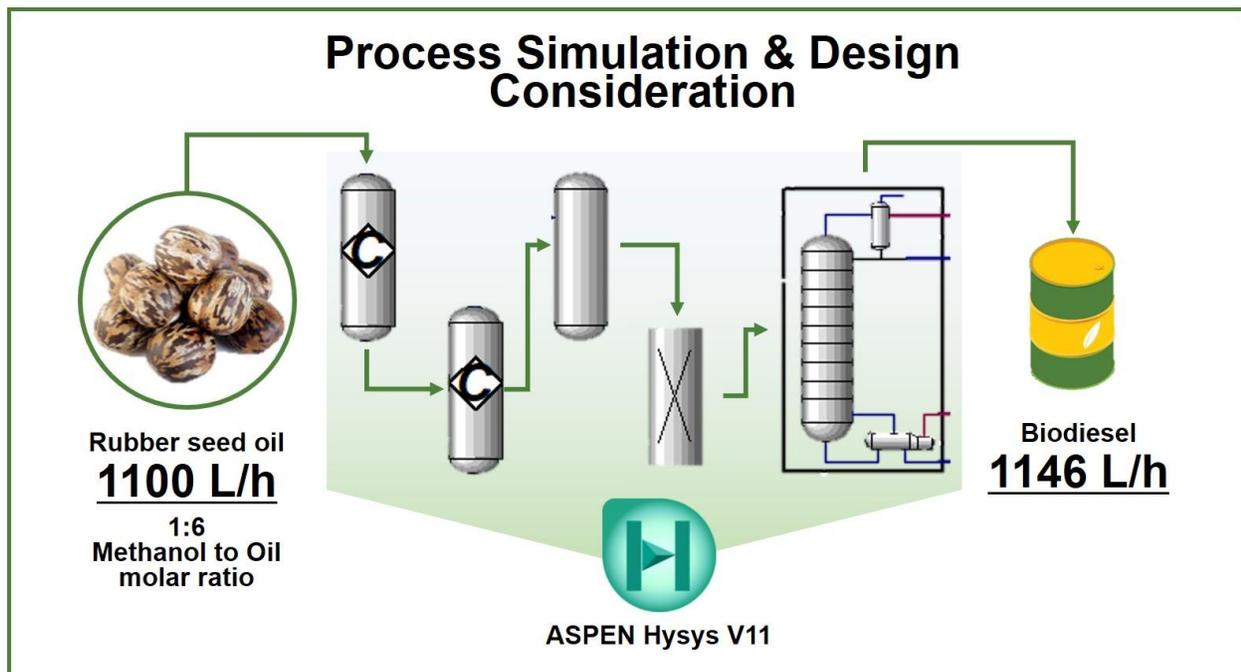
**Figure 602.** Biodiesel yield from rubber seed oil
