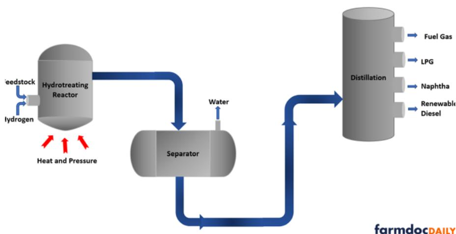
**Figure 257.** HVO renewable diesel production process
