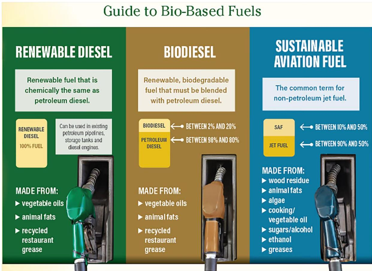
Figure 268. Renewable diesel, biodiesel, and SAF comparison
