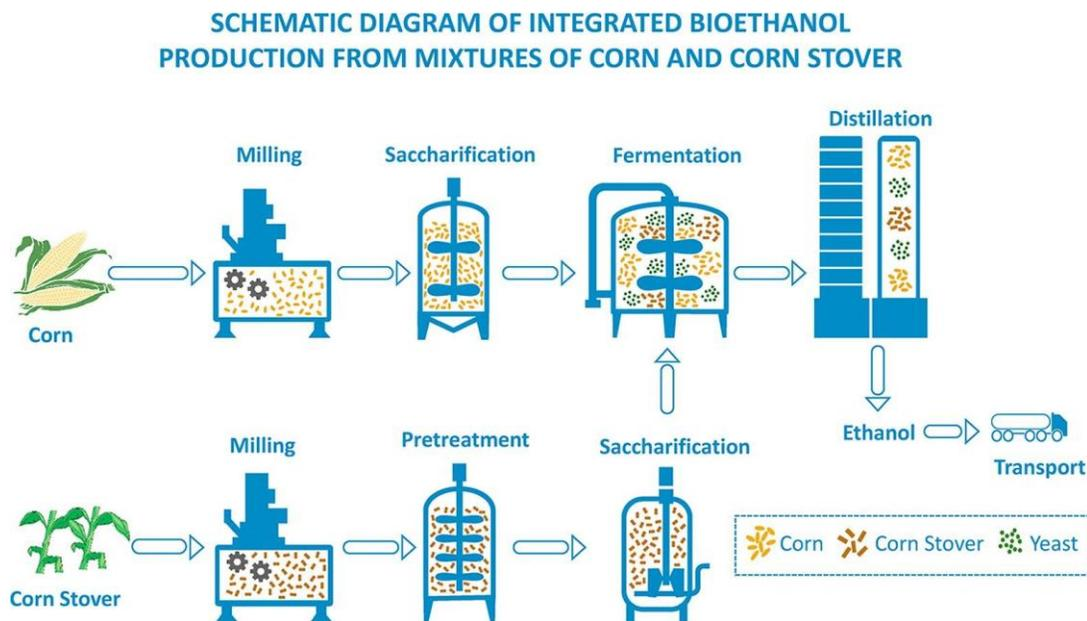
**Figure 557.** Bioethanol production process from corn grain and stover
