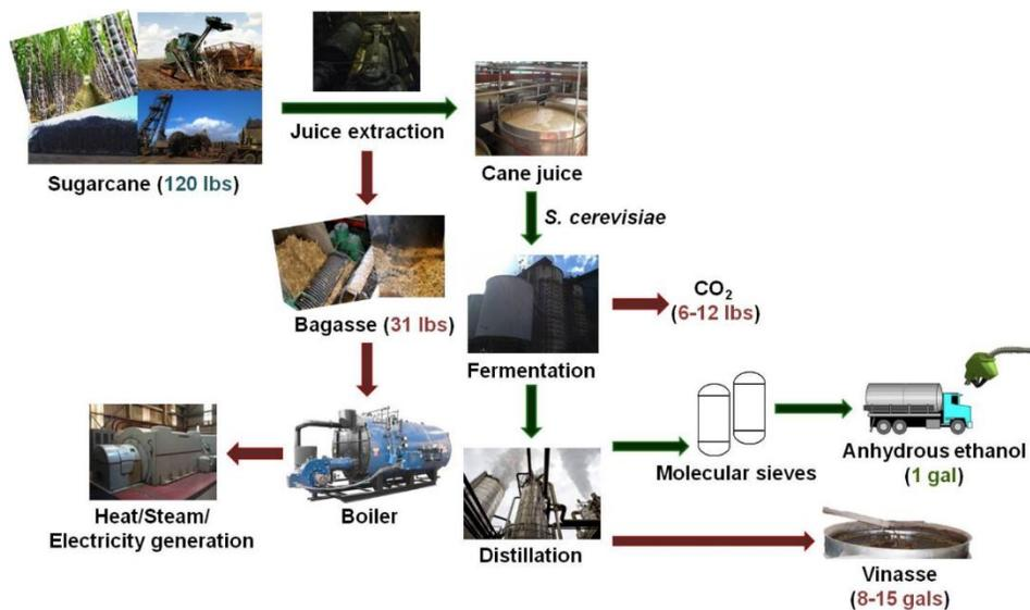
**Figure 368.** Biofuel production process from sugarcane juice
