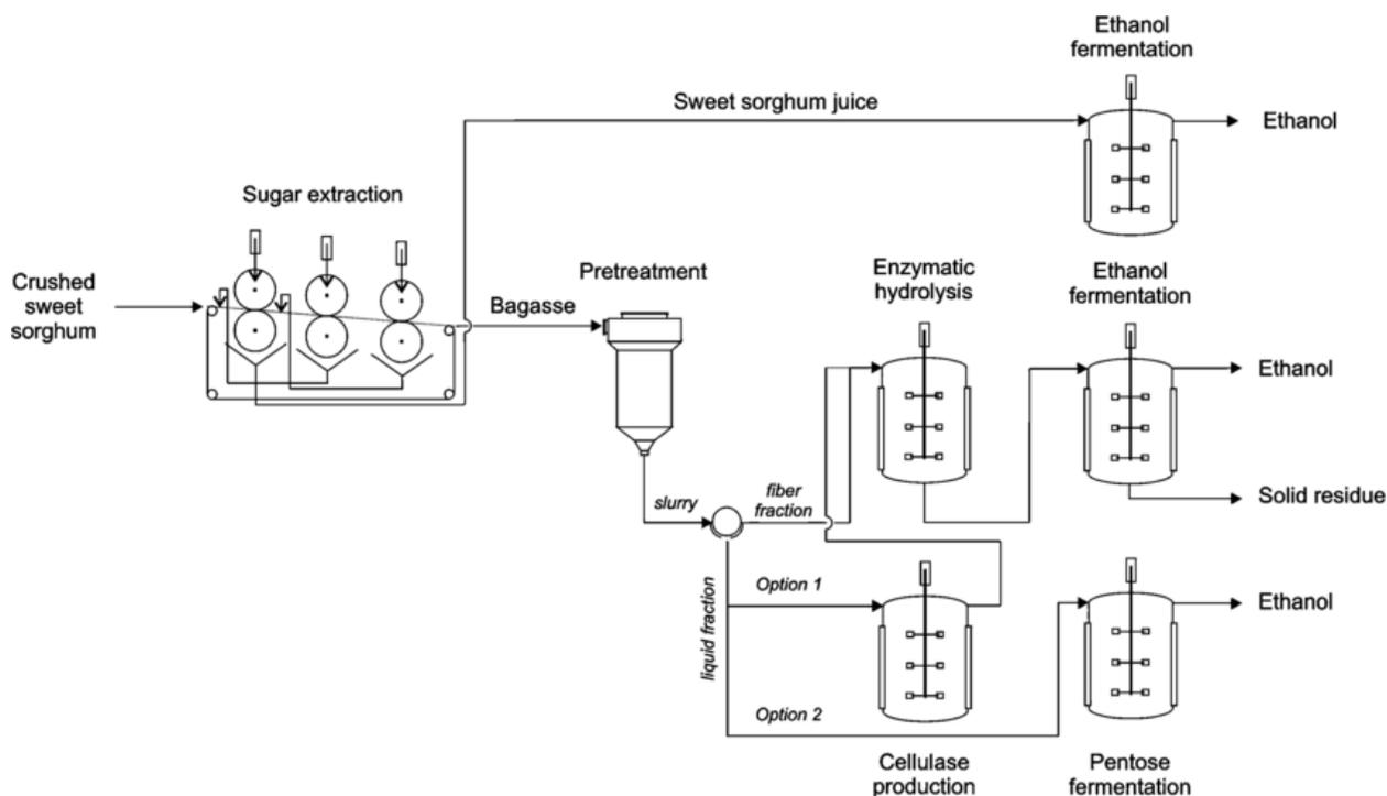
**Figure 468.** Process to make bioethanol from sorghum feedstock
