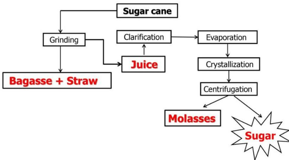
**Figure 335.** Sugarcane Processing By-products
