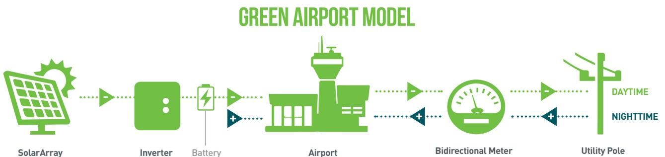
▶ Excess energy not used by airport that goes back to the grid    ▶ Energy used by airport from the grid or battery
