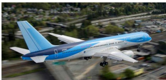
**Figure 3.** B757 EcoDemonstrator With AFC on Vertical Fin<sup>3</sup>
