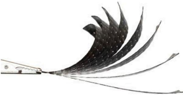
**Figure 7.** Programmable Adaptable Carbon Fiber (laboratory test coupon).
