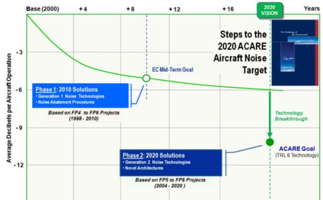
Figure 1. Steps to ACARE 2020 noise target.
