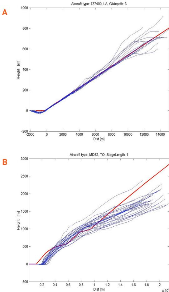
**Figure 6.** Flight Profiles (Height Via Distance) Observed In Operation (blue lines) In Comparison With Balanced Prediction (red lines): A – Arrival; B – Departure.<sup>10</sup>
