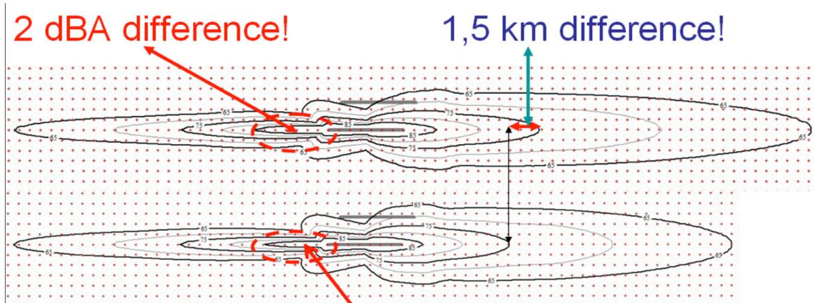
**Figure 8b.** IsoBellaResults for B-737-400Noise Contours (approach/landing and take-off/climbing) are Higher When Using Input Data for Flight Parameters Observed in Operations; and Lower for Balanced Input Data for Flight Parameters
