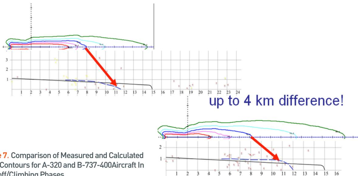
**Figure 7.** Comparison of Measured and Calculated Noise Contours for A-320 and B-737-400 Aircraft In Take-off/Climbing Phases.
