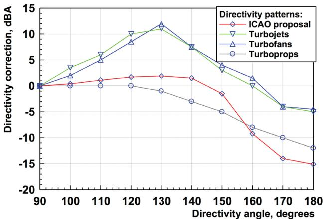
**Figure 1.** Generalized Directivity Corrections for Characteristic Engine Types.
