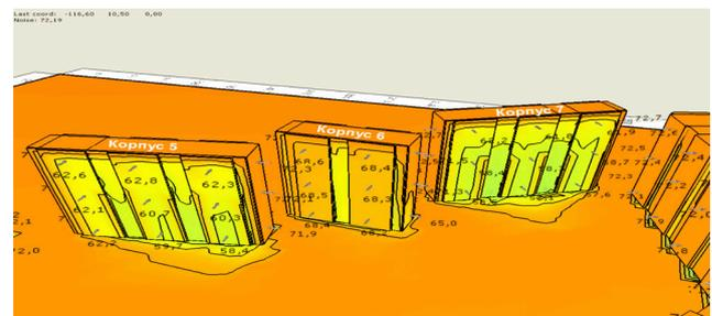
**Figure 4b.** Cartographic Visualized Assessment of the Noise Situation of Protected Facilities Exposed to Maximum Aircraft Noise Levels at Night. Perspective Projection of the Noise Picture of the North-east Facades of Building #5 and Adjacent Area.
