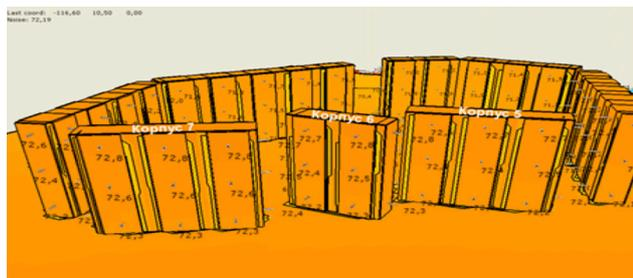
**Figure 4a.** Cartographic Visualized Assessment of the Noise Situation of Protected Facilities Exposed to Maximum Aircraft Noise Levels at Night. Perspective Projection of the Noise Picture of the South-west Facades of Building #5.
