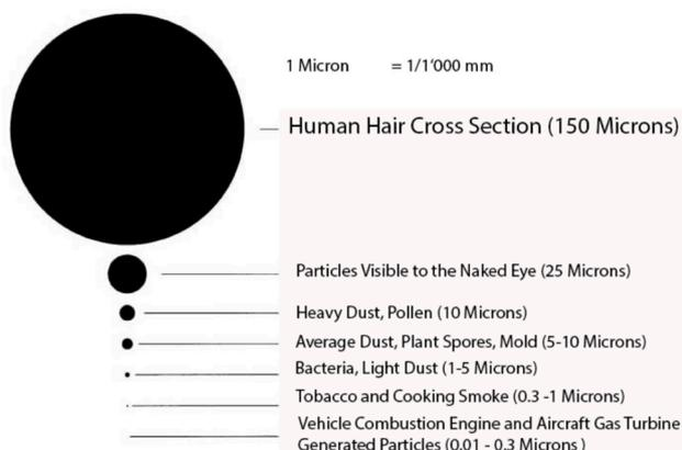
**Figure 1.** Comparison of Particle Sizes from Different Sources.
