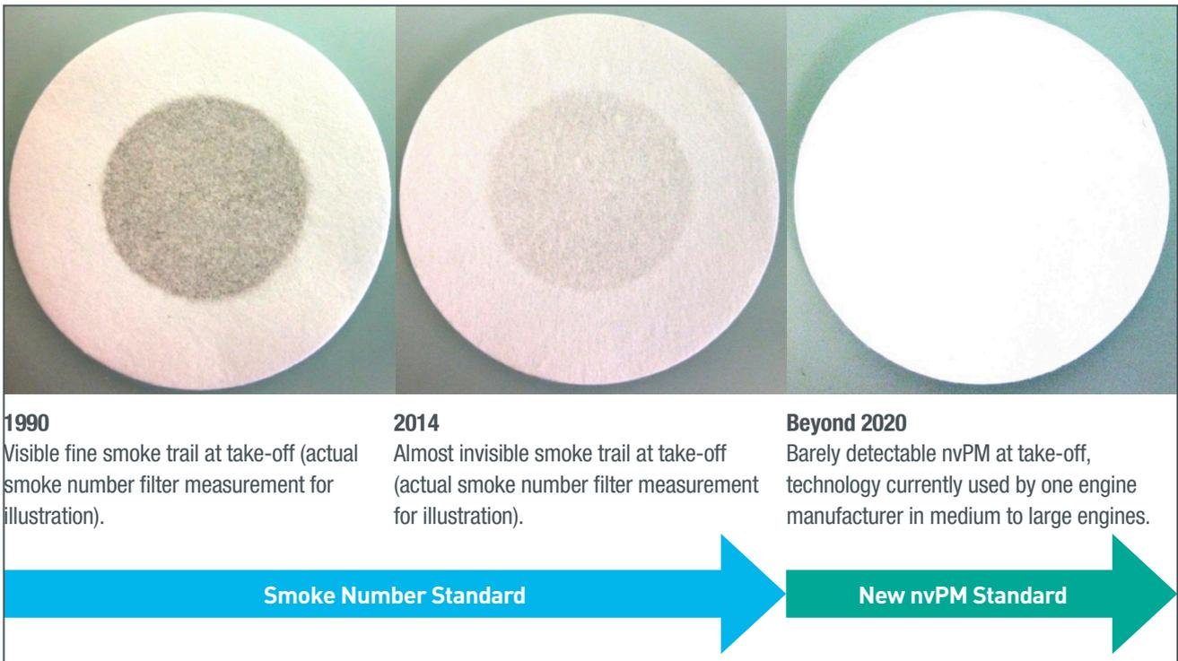
**Figure 7.** From smoke number standard to the new nvPM standard.
