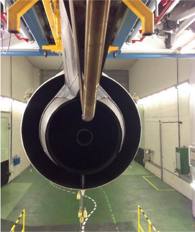
**Figure 2.** Turbfan Engine Seen From Behind With Tube of a Sampling Probe.
