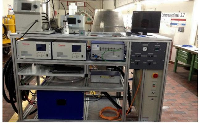
**Figure 3.** Sections of the Swiss nvPM Sampling and Measurement System With Added Particle Sizing Instrumentation. (Sections 4 and 5 in Figure 4).
