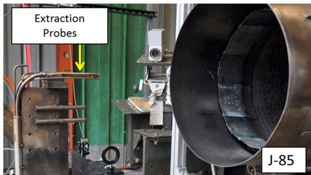
Figure 5. The VARIAnT Probe System (Courtesy of AEDC).
